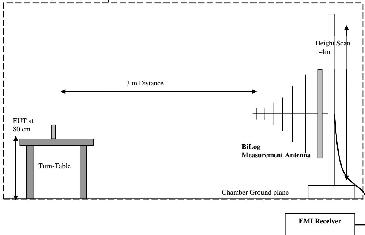
Radiated Emissions Test Setup Above 1GHz Measurements
