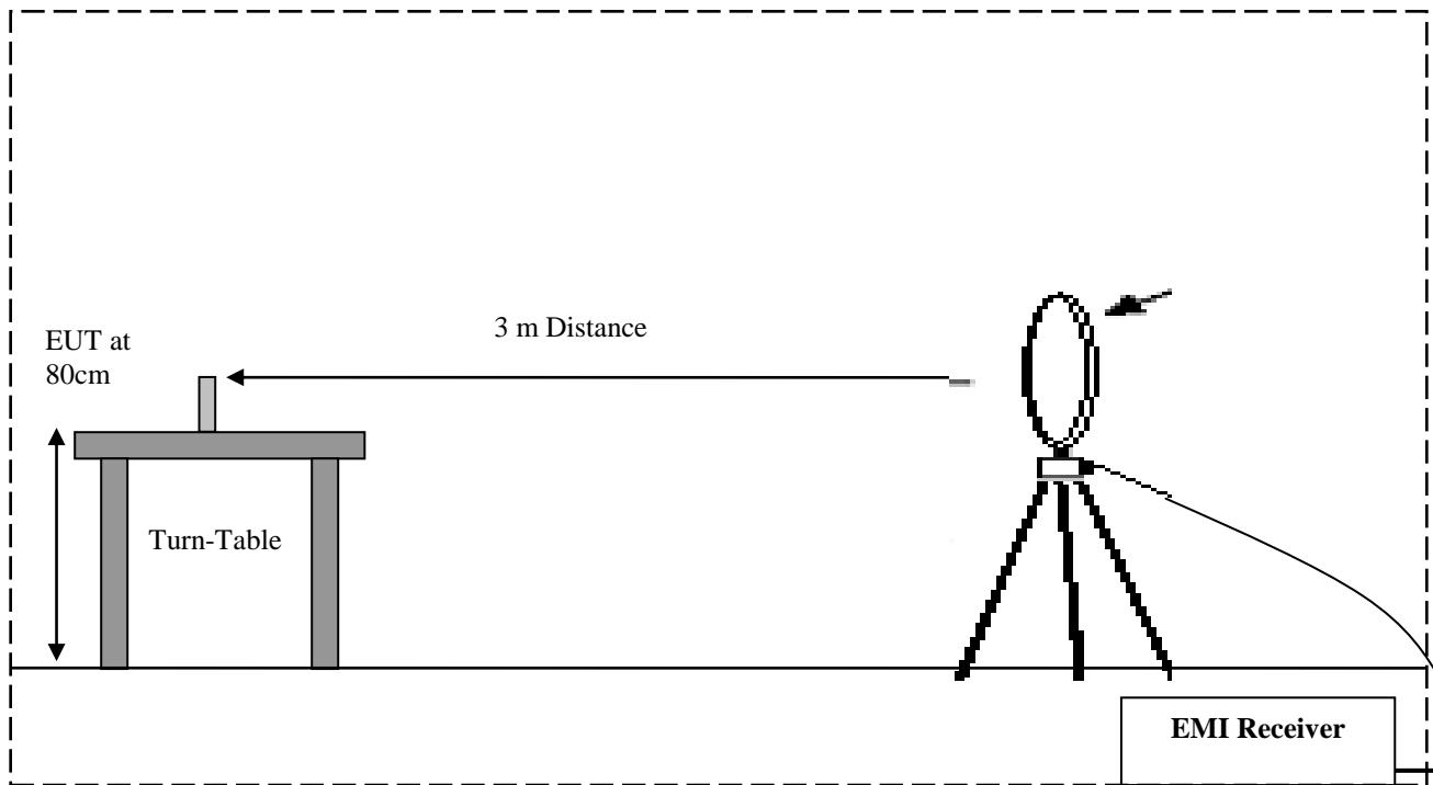
Radiated Emissions Test Setup 30MHz-1GHz Measurements
