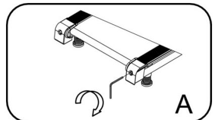
1. Place treadmill on a level surface and run at full speed. If the belt drifts to the right, pull out the switch, turn the right adjusting bolt 1/4 turn clockwise, then start running until centering the belt.
