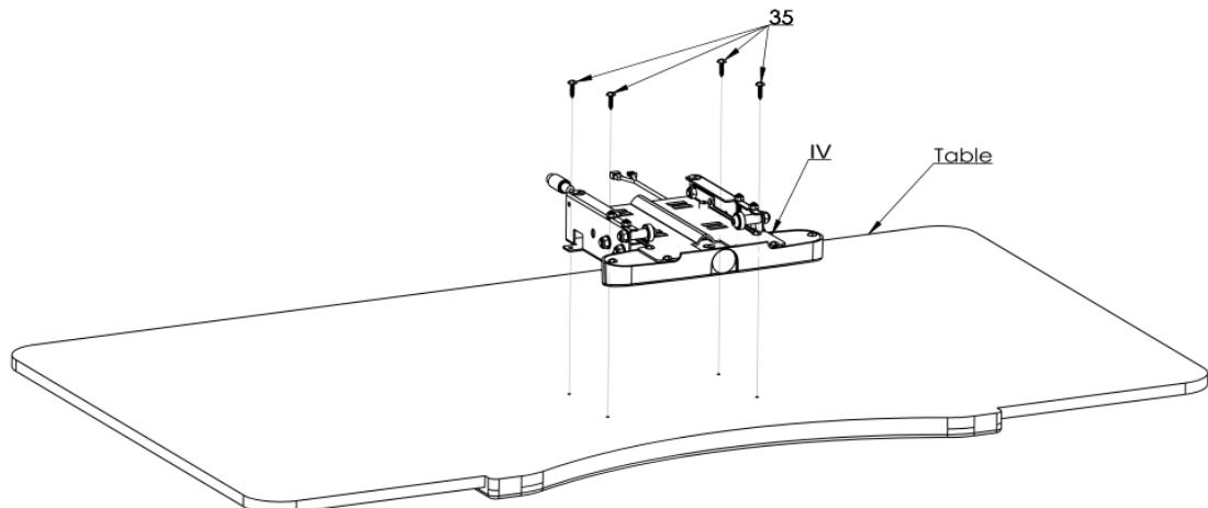
*Remarks: Adjust the tension of the console set on the rails by the 4 pieces of screws as the arrows point in the below picture.*
