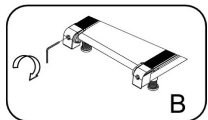
2. If the belt drifts to the left, pull out the switch, turn the left adjusting bolt 1/4 turn clockwise, then start running until centering the belt. **PICTURE - B**
