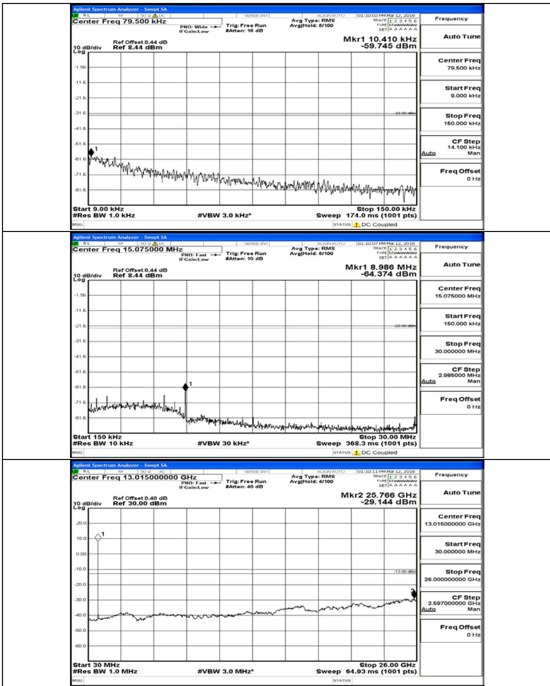
Channel Bandwidth: 10 MHz\_HCH\_QPSK\_1RB#0
