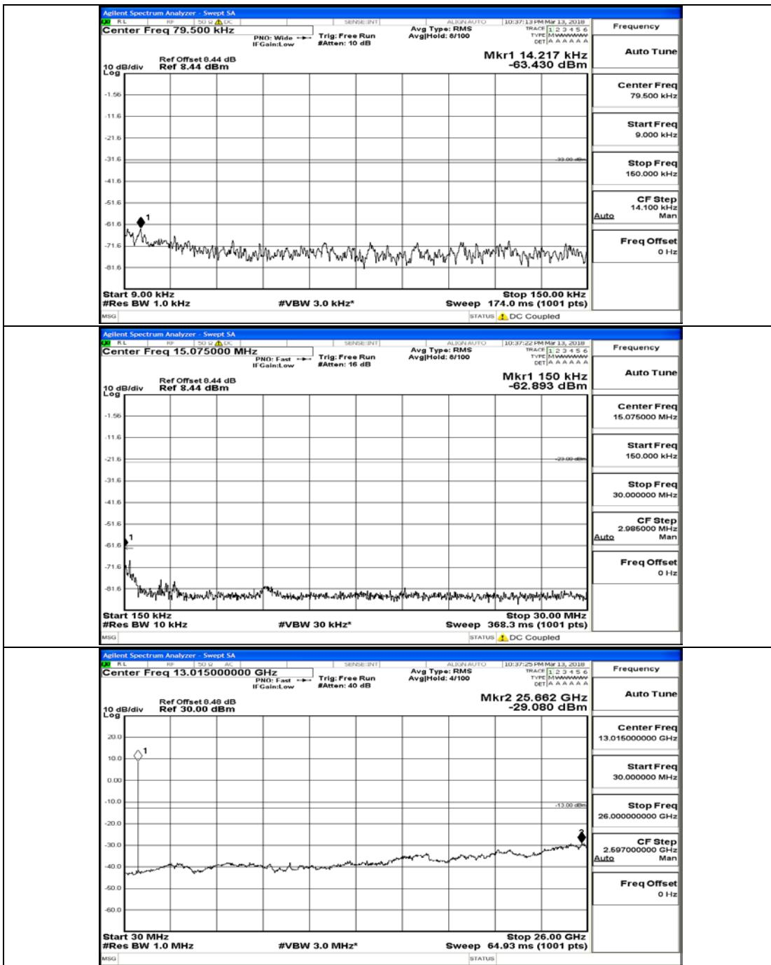
(Channel Bandwidth: 1.4 MHz)\_HCH\_QPSK\_1RB#0
