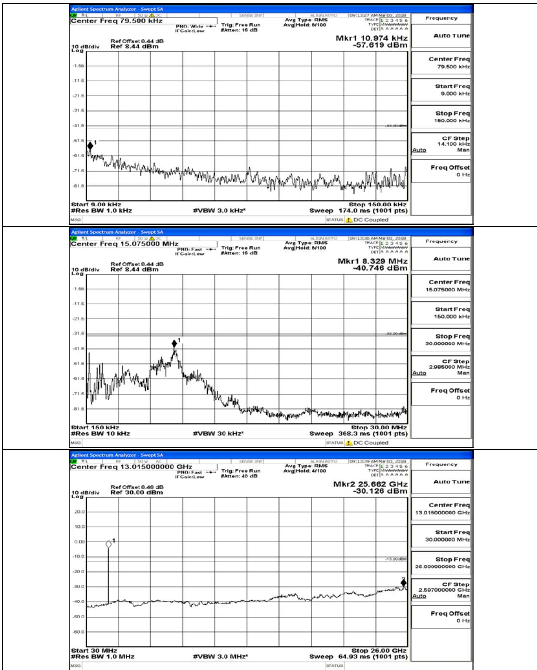
(Channel Bandwidth: 1.4 MHz)\_HCH\_16QAM\_1RB#0
