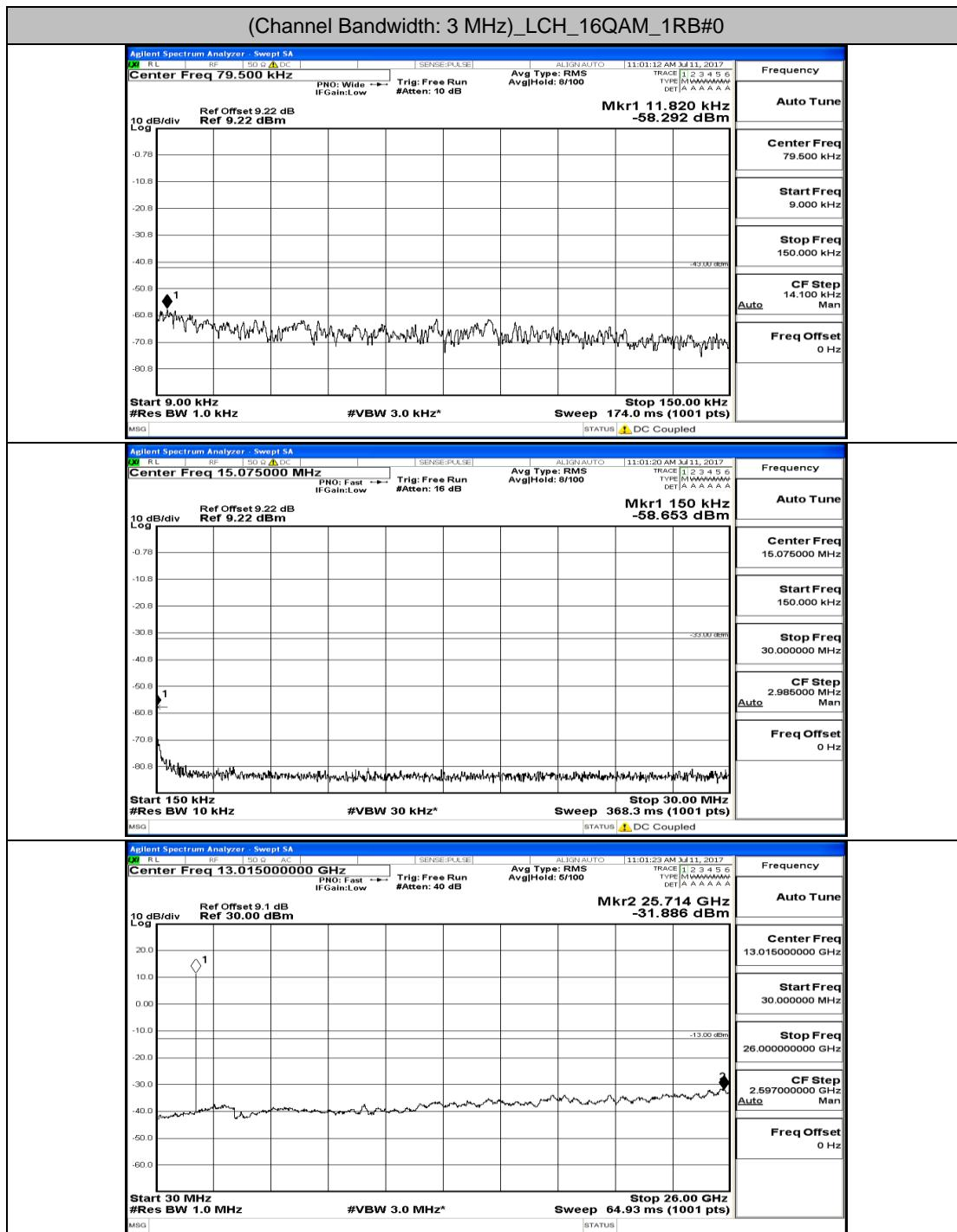
(Channel Bandwidth: 3 MHz)\_MCH\_16QAM\_1RB#0
