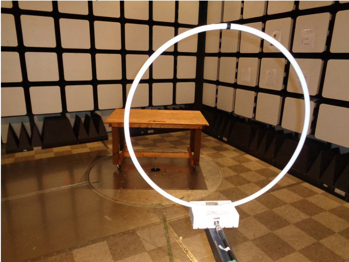
Figure 6 – Radiated Emissions below 30 MHz
