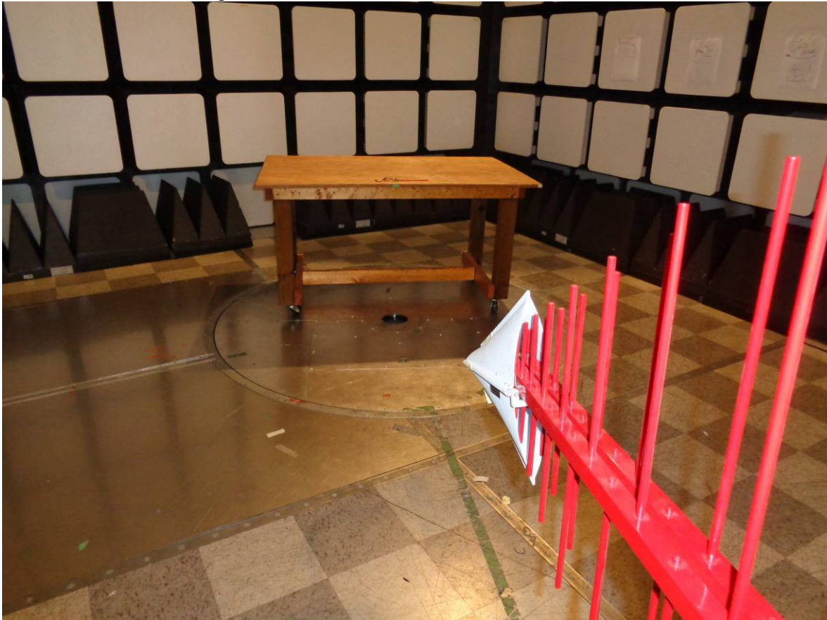
Figure 7 – Radiated Emissions 30MHz to 1GHz
