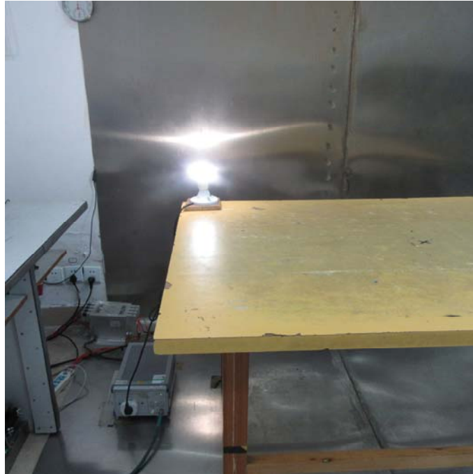
Conducted Disturbance Test Setup Side View
