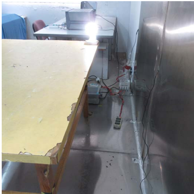
Conducted Disturbance Test Setup Side View
