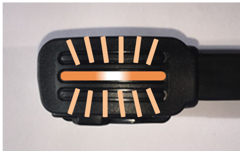
Figure 14 Fast Orange LED, UTP Fob Training Failed
