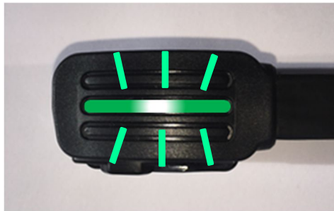
Figure 9 Slow Green LED Blink UTP 1.0 Configuring Correctly
