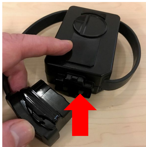
Fasten OBDII connector to enclosure
