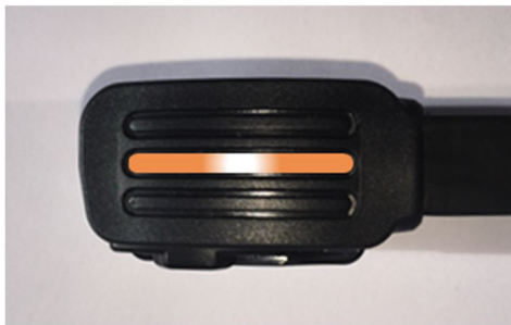
Figure 18 Solid Orange LED Indicates Fob Trained
