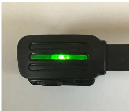
Figure 4 OBD Solid green LED indicates successful in-fleet
