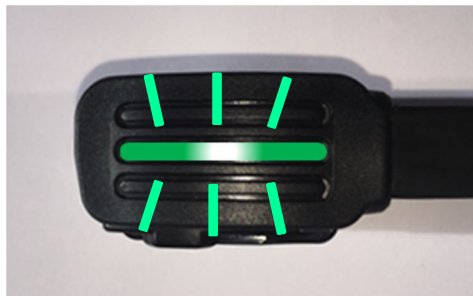
Figure 3 Slow Green LED Blink UTP 1.0 Configuring Correctly
