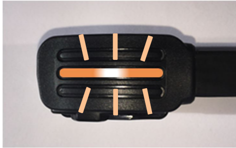
Figure 13 Slow Orange LED, UTP Successfully Trained as Key Fob
