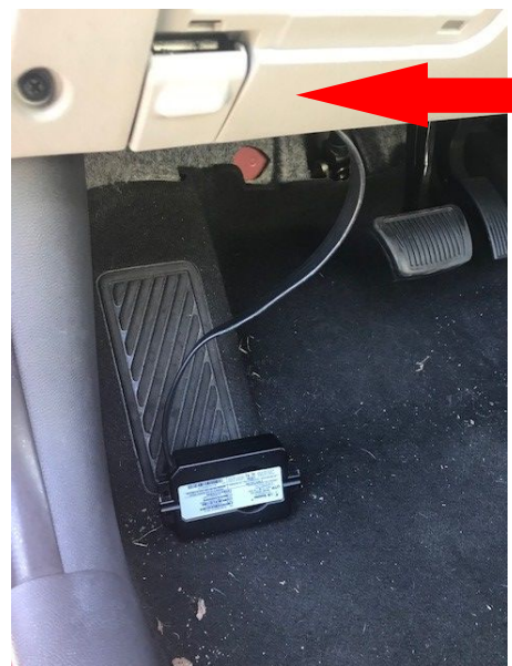
UTP 1.0 plugged into OBD-II port (Port Left - Facing Out Right – Port Facing Down)
