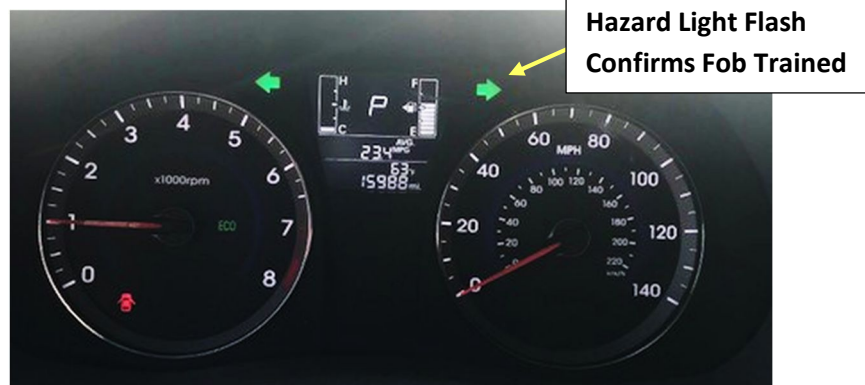
Figure 17 Observe Vehicle Hazard Light Flash
