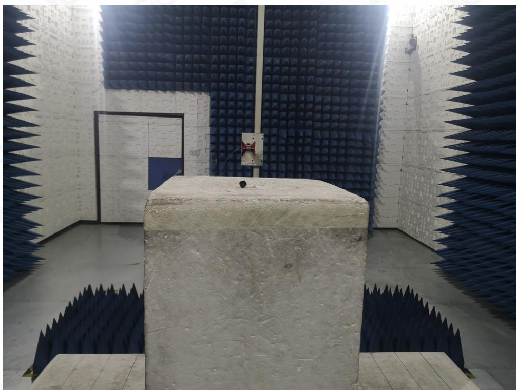
RADIATED EMISSION TEST SETUP ABOVE 1GHZ
