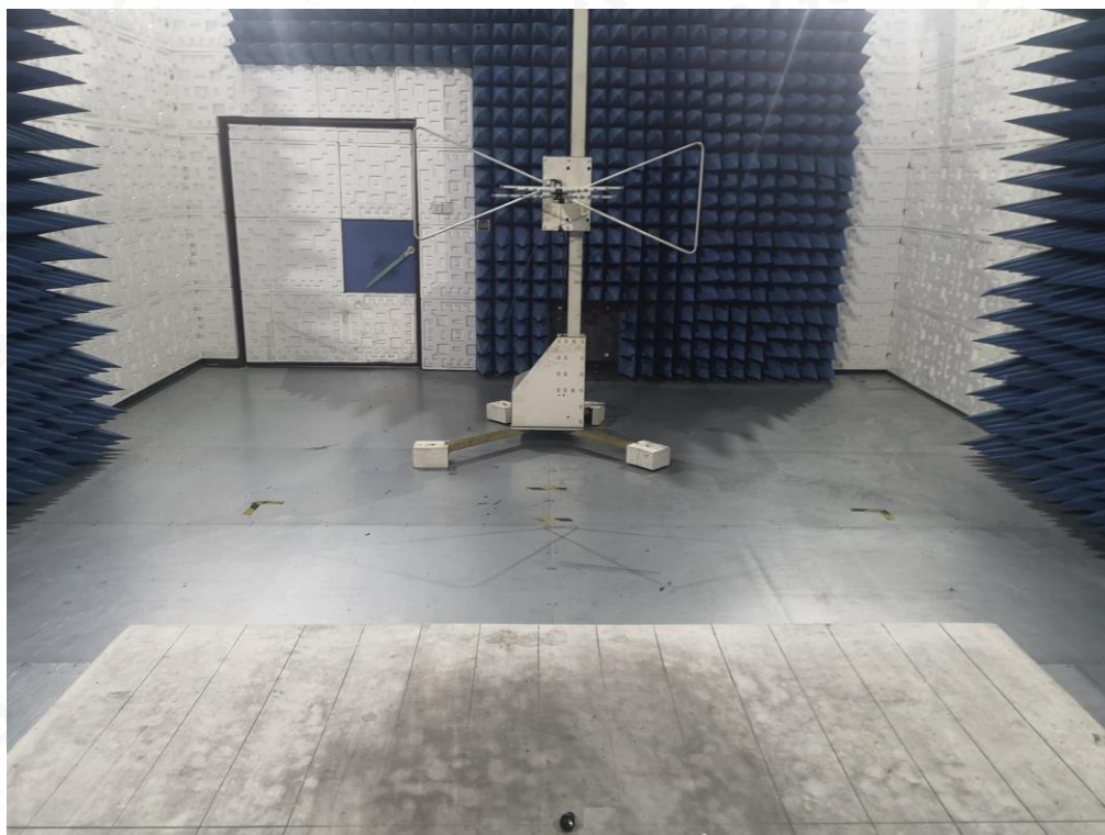
RADIATED EMISSION TEST SETUP ABOVE 1GHZ
