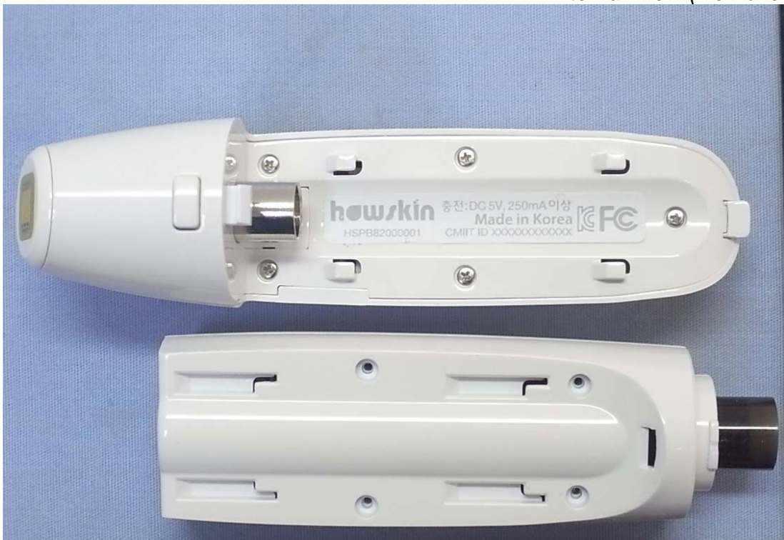
Figure 4 Internal View (Removed Cover)
