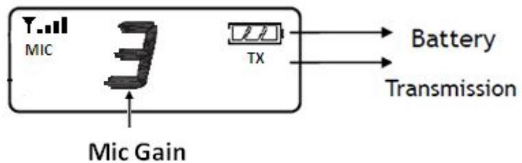
4. Press “Tx(PPT)” Key to enable or disable the RF transmit,
