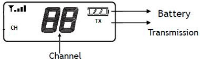
2. Press "Channel Up/Down" to change the channel: 0-99 (Freq:910-920Mhz,100khz Channel Spacing );
