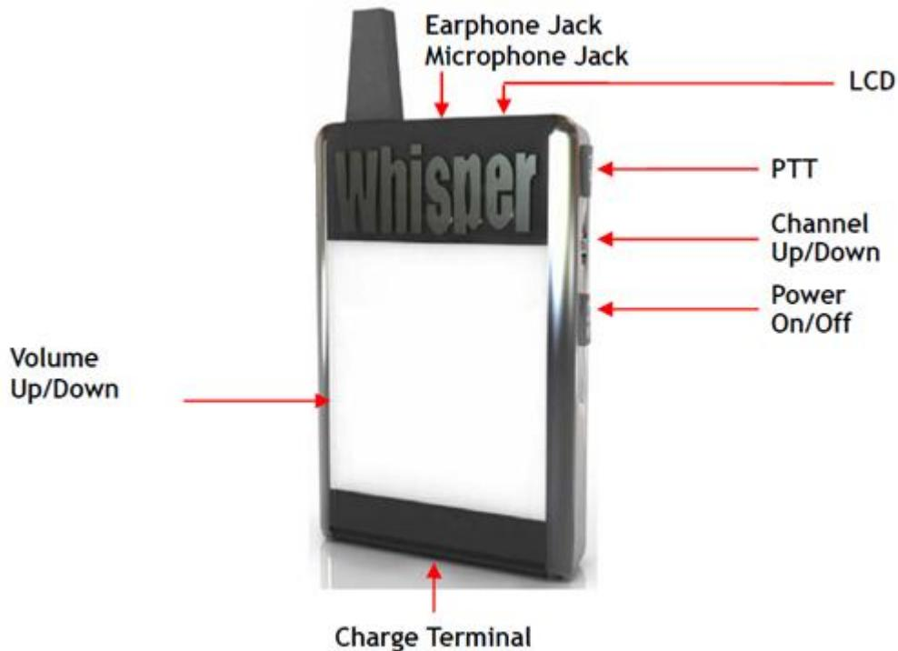
1. Press and Hold the "Power On/Of" Key , System boot , Press and Hold the "Power On/Of" Key , System boot (At the same time the Buzzer will ring inside the machine)
