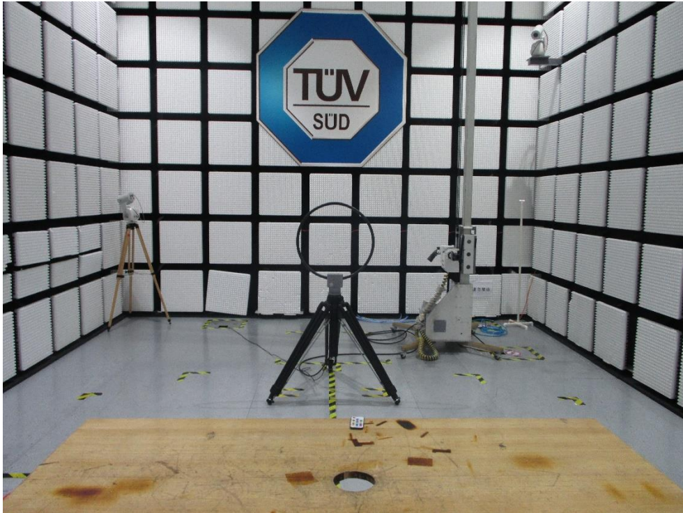
Radiated Emission Setup 9kHz ~ 30MHz
