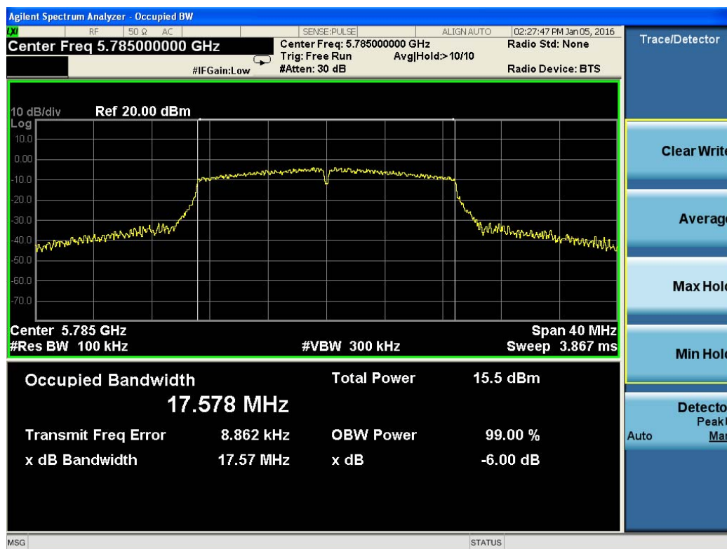
Test Plot For 802.11n(HT20)-6dB BW-5785M
