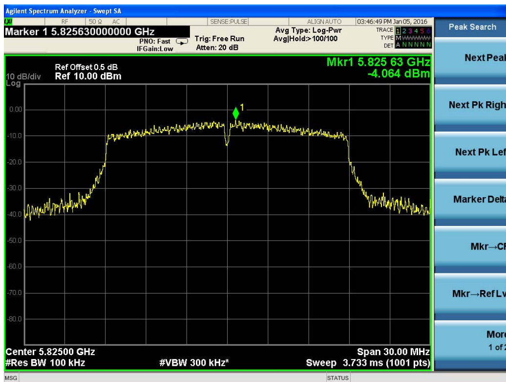
Test Plot For 802.11n(HT20)-5825M
