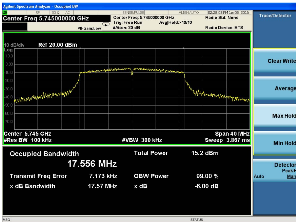
Test Plot For 802.11n(HT20)-6dB BW-5745M
