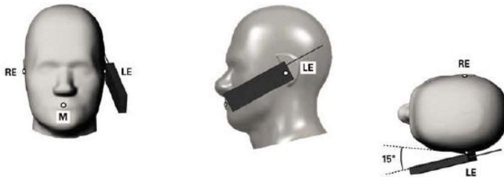
Fig.11.4 Illustration for Tilted Position
