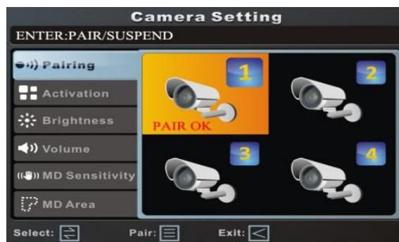
Short press “ $\Rightarrow$ ” icon button (selection key), select another camera, repeat the above operation, complete the pairing operation of the host and other cameras.
