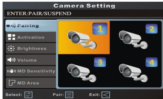
Then short press “≡” icon button (menu key), the host and the 1<sup>st</sup> camera start pairing, at this time, immediately short press the pairing key on the power line of the 1<sup>st</sup> camera (please ensure that camera is connected with a DC 5V 1A power. If you are not sure which camera is the 1<sup>st</sup> camera, you can short press pairing key of each camera), as shown below.
