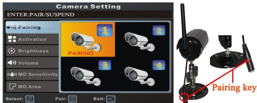
If the "pairing" menu interface of host shows "pairing time out", please repeat the above operation again for pairing. The success of the pairing menu interface for 1<sup>st</sup> camera is as shown below.
