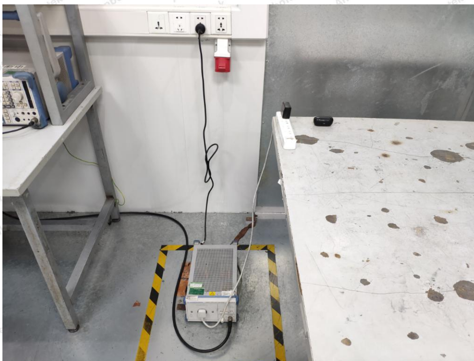
Photo of Conducted Emission Measurement
