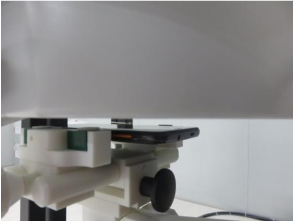
10mm body-worn Front Side Setup Photo(hotspot)
