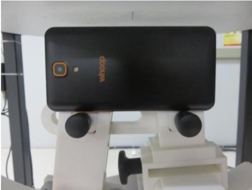
10mm body-worn Right Side Setup Photo(hotspot)
