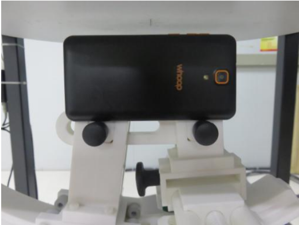
10mm body-worn Left Side Setup Photo(hotspot)
