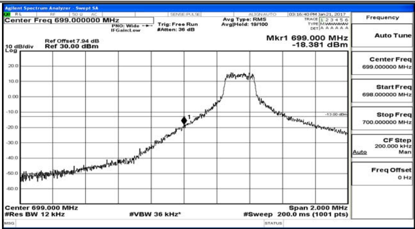
(Channel Bandwidth: 5 MHz)_LCH_QPSK_25RB#0
