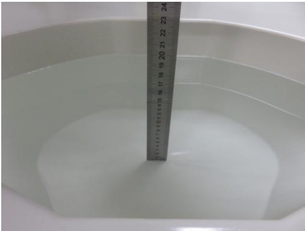
Photograph of the depth in the Body Phantom (5000MHz, 16.3cm depth)
