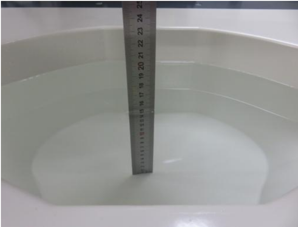
Photograph of the depth in the Body Phantom (2450MHz, 15.6cm depth)
