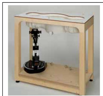
The bottom plate contains three pair of bolts for locking the device holder. The device holder positions areadjusted to the standard measurement positions in the three sections. A white cover is provided to tap thephantom during off-periods to prevent water evaporation and changes in the liquid parameters. On thephantom tip, three reference markers are provided to identify the phantom position with respect to therobot.
