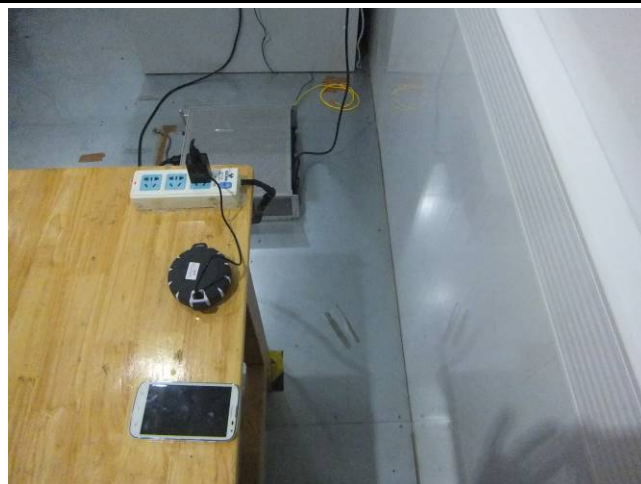
Conducted Emissions Test Setup – Side View
