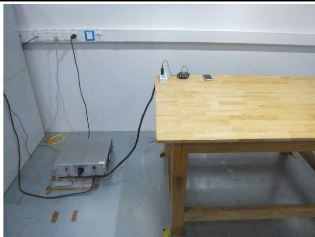
Conducted Emissions Test Setup – Front View
