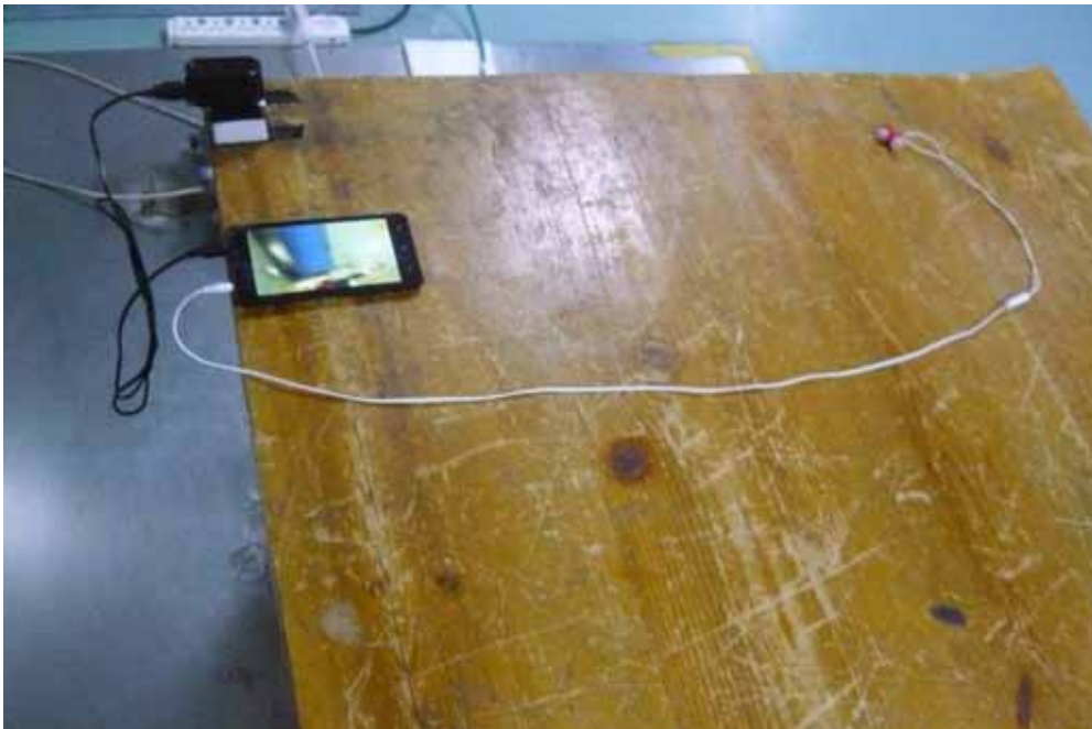
Conducted Emission-Rear View
