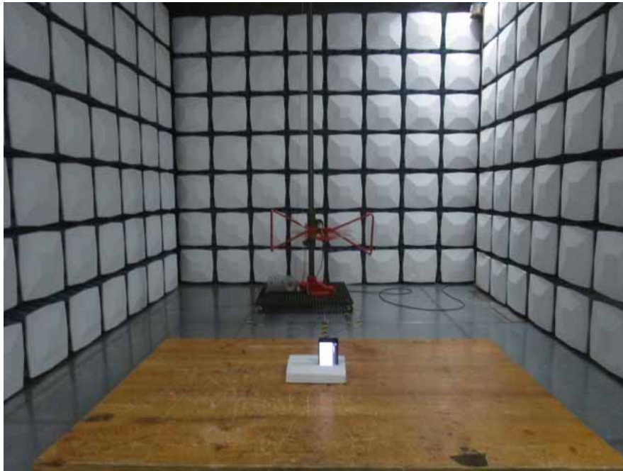
Radiated Emission View (Below 1GHz)
