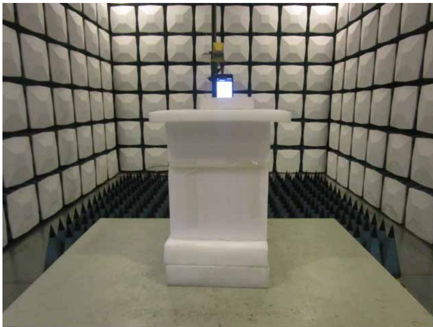
Radiated Emission View (Above 1GHz)
