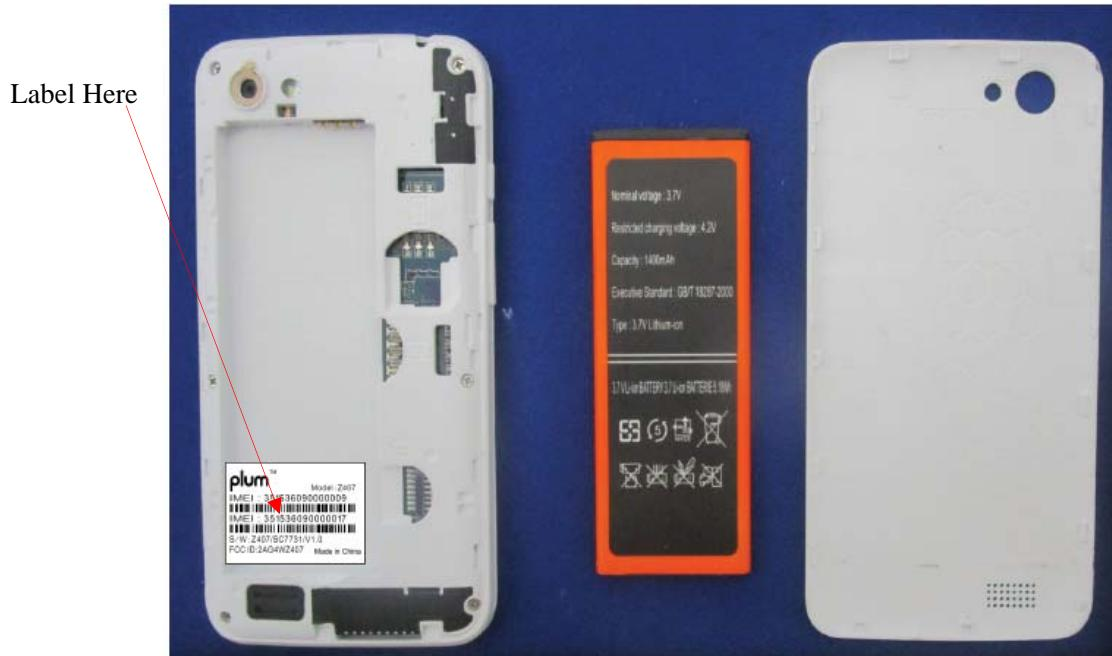
The label shown shall be permanently affixed at a conspicuous location on the device and be readily visible to the user at the time of purchase (Labeling requirements per 2.925)
