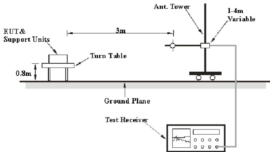
The radiated emission tests were performed in the 10-meter chamber test site, using the setup accordance with the ANSI C63.10-2013. The specification used was the FCC Part Subpart C limits.
