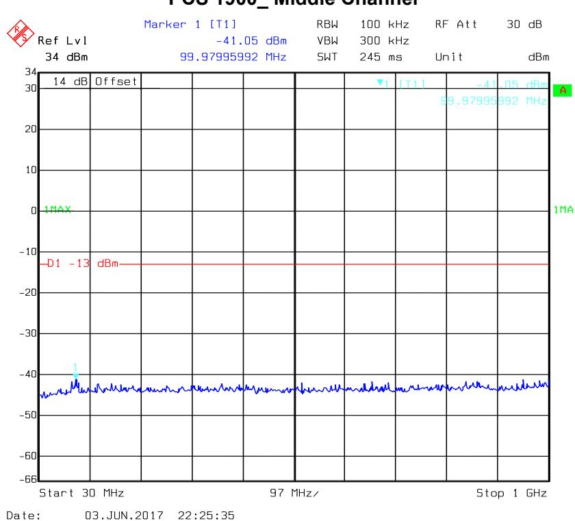
Fundamental test with band rejection filter
