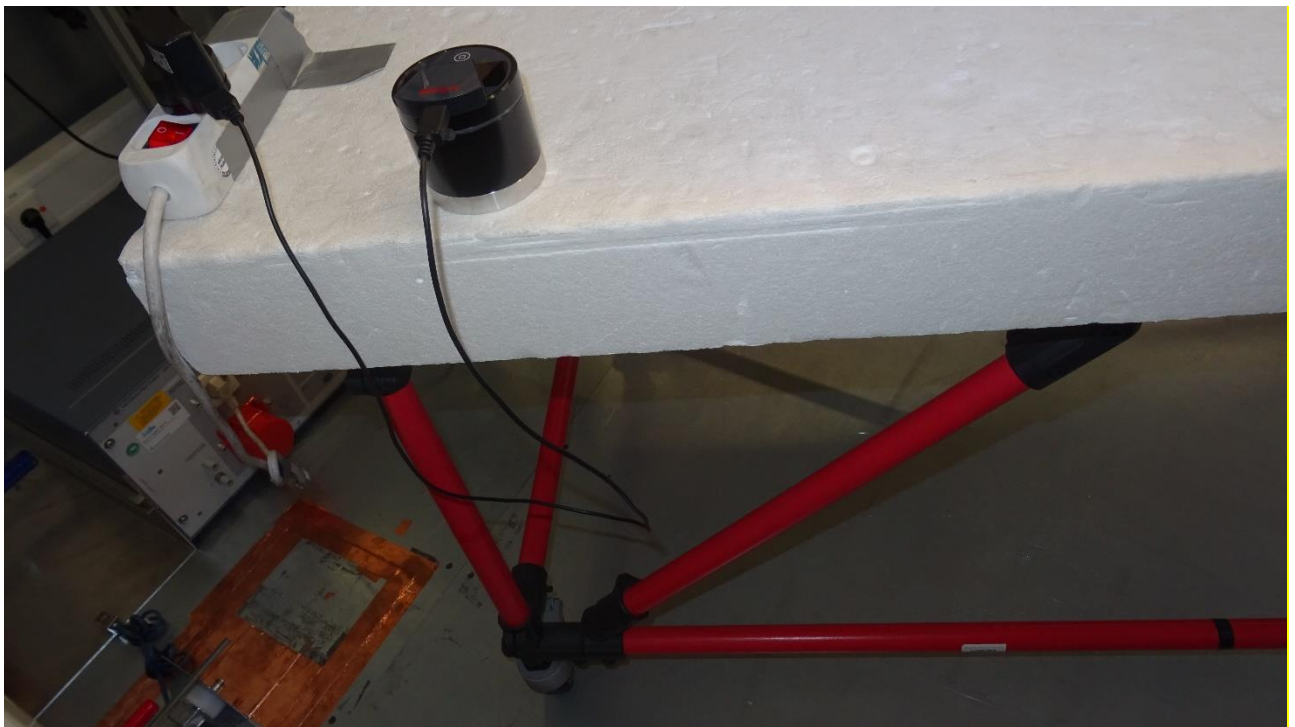
Picture 8: Test setup AC power line conducted emissions (rear view), charging mode
