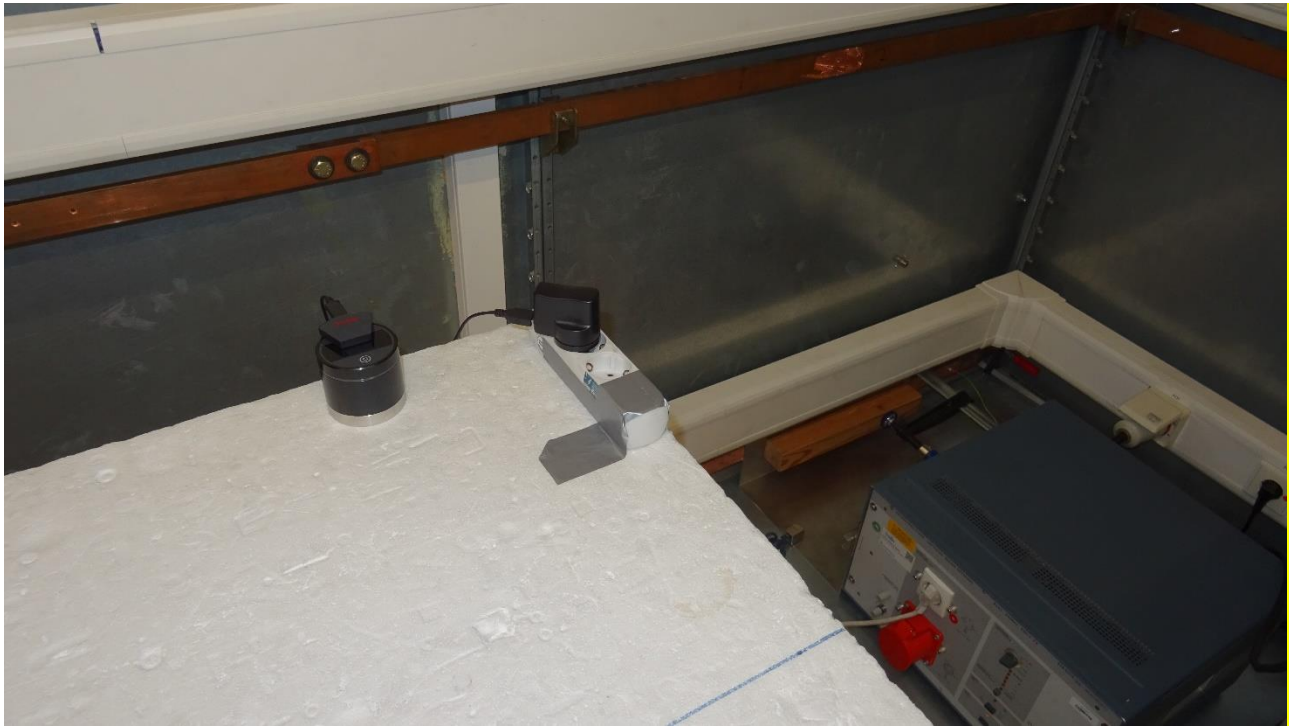
Picture 7: Test setup AC power line conducted emissions (front view), charging mode
