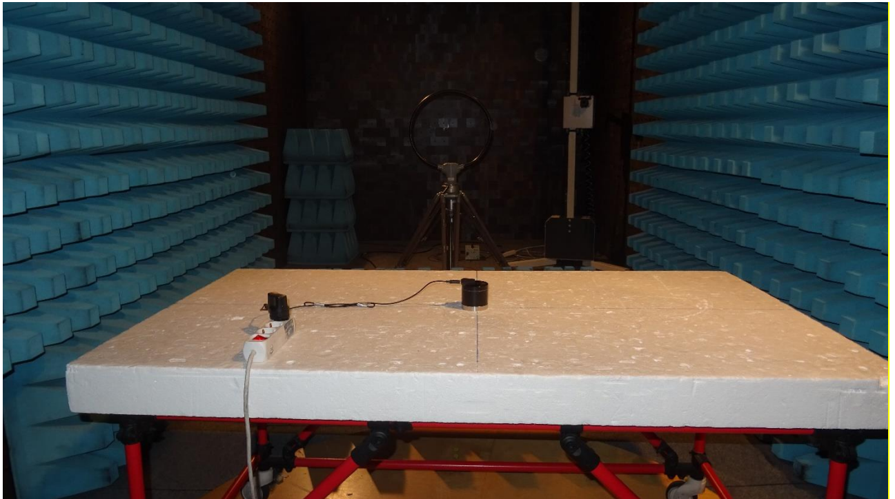
Picture 1: CDC, test setup radiated emission test 9 kHz - 30 MHz (front view), charging mode
