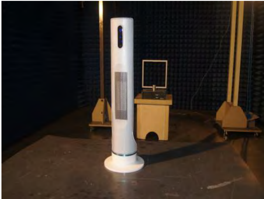
Photograph 2: Set-up for Radiated Spurious Emission (30MHz ~ 1GHz)
