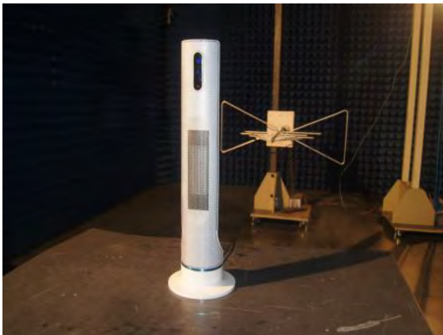
Photograph 2: Set-up for Radiated Spurious Emission (30MHz ~ 1GHz)
