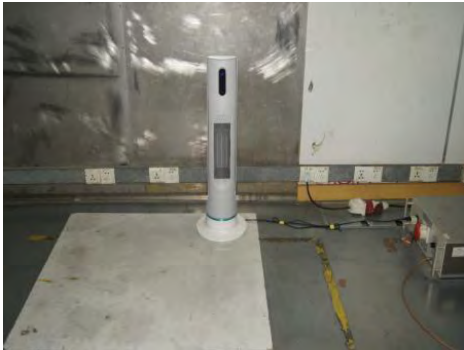
Photograph 6: Set-up for Radiated Emission, below 1GHz
