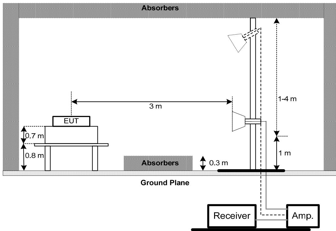
(C) For Radiated Emissions Below 30MHz
