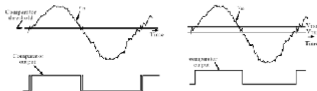
Picture 11-3 (a) Ordinary comparator noise impact (b) Hysteresis added comparator noise impact
