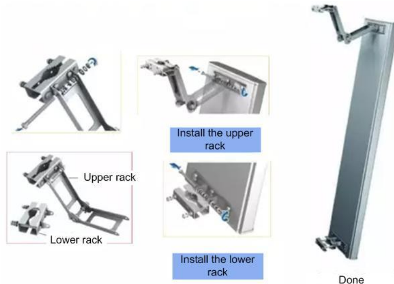
Figure 3-5 Assembling Procedure of Directional Antennas
