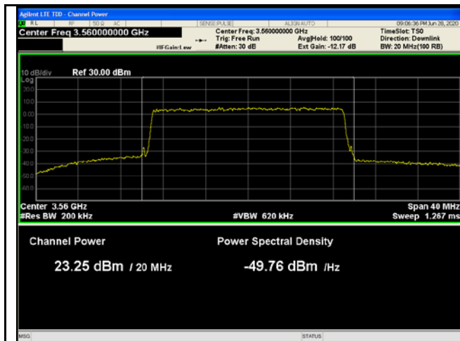
20MHz Full - Low CH QPSK
