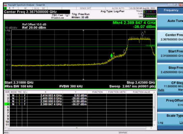
,Plot 2,Band Edge-802.11n(HT20) ,2437MHz,Ant1
