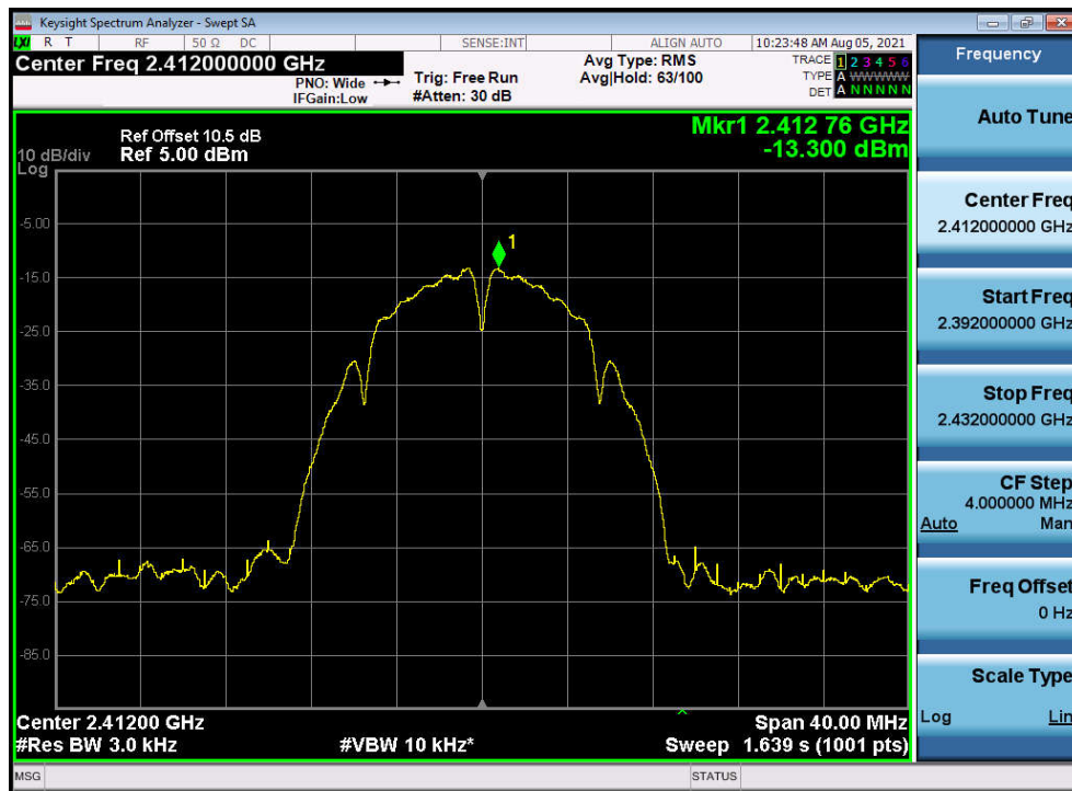
Power spectral density-802.11b ,2412MHz,Ant0
