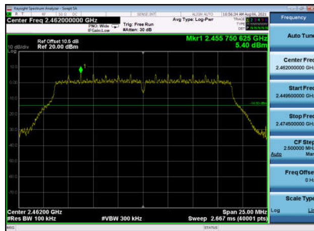
,Plot 1,Reference Level-802.11n(HT20) ,2462MHz,Ant1
