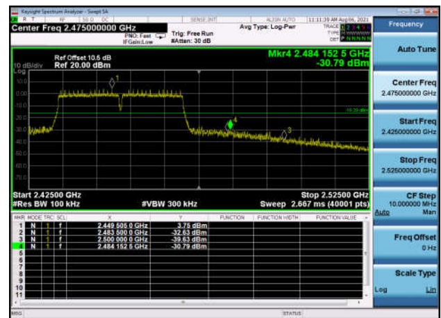
,Plot 2,Band Edge-802.11n(HT40) ,2452MHz,Ant1
