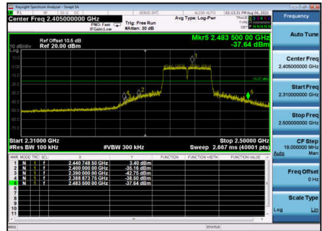
,Plot 2,Band Edge-802.11n(HT40) ,2452MHz,Ant1
