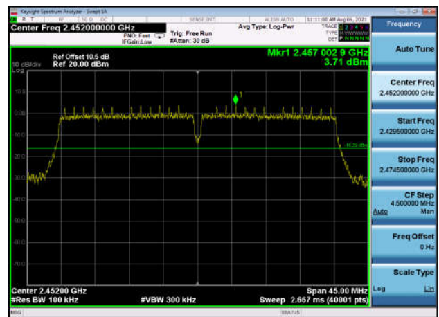
,Plot 1,Reference Level-802.11n(HT40) ,2452MHz,Ant1
