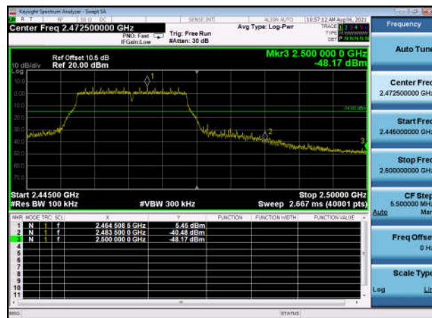
,Plot 2,Band Edge-802.11n(HT20) ,2462MHz,Ant1
