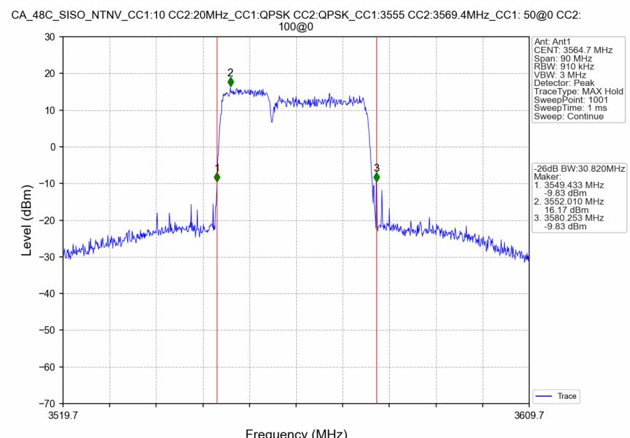
CA\_48C\_SISO\_NTNV\_CC1:10 CC2:20MHz\_CC1:QPSK CC2:QPSK\_CC1:3675.6 CC2:3690MHz\_CC1: 50@0 CC2:
