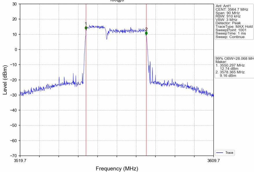
CA\_48C\_SISO\_NTNV\_CC1:10 CC2:20MHz\_CC1:QPSK CC2:QPSK\_CC1:3675.6 CC2:3690MHz\_CC1: 50@0 CC2: 100@0
