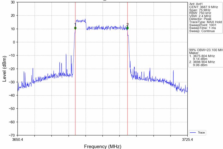
CA\_48C\_SISO\_NTNV\_CC1:10 CC2:20MHz\_CC1:QPSK CC2:QPSK\_CC1:3555 CC2:3569.4MHz\_CC1: 50@0 CC2: 100@0
