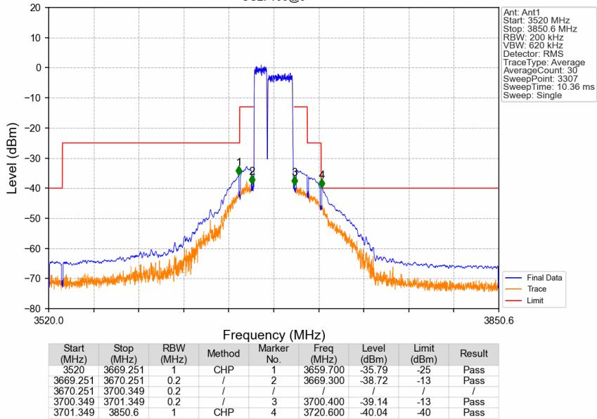
CA\_48C\_SISO\_NTNV\_CC1:10 CC2:20MHz\_CC1:16QAM CC2:16QAM\_CC1:3675.6 CC2:3690MHz\_CC1: 50@0 CC2: 100@0
