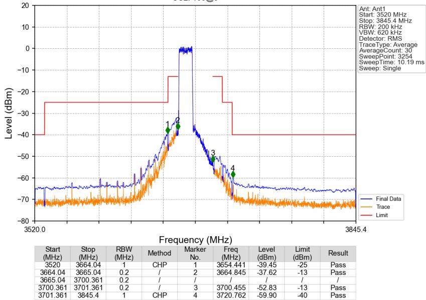
CA\_48C\_SISO\_NTNV\_CC1:15 CC2:20MHz\_CC1:16QAM CC2:16QAM\_CC1:3672.9 CC2:3690MHz\_CC1: 75@0 CC2: 100@0
