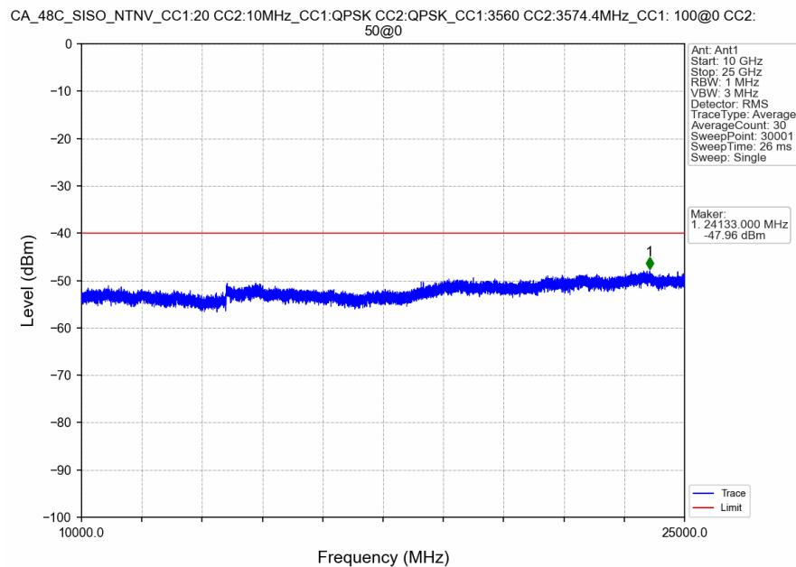
CA\_48C\_SISO\_NTNV\_CC1:20 CC2:10MHz\_CC1:QPSK CC2:QPSK\_CC1:3560 CC2:3574.4MHz\_CC1: 100@0 CC2:
