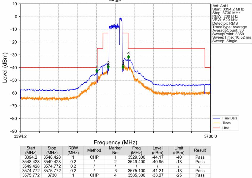
CA\_48C\_SISO\_NTNV\_CC1:20 CC2:5MHz\_CC1:QPSK CC2:QPSK\_CC1:3560 CC2:3571.7MHz\_CC1: 100@0 CC2:
