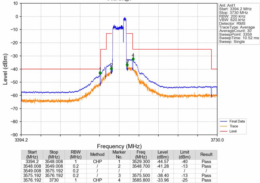
CA\_48C\_SISO\_NTNV\_CC1:20 CC2:5MHz\_CC1:16QAM CC2:16QAM\_CC1:3560 CC2:3571.7MHz\_CC1: 100@0 CC2: 25@0
