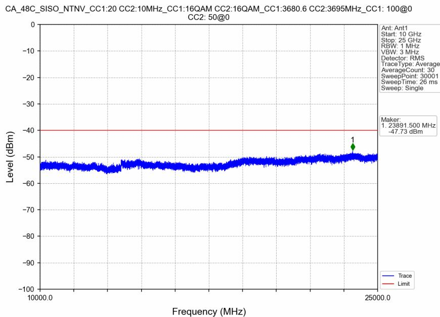
CA\_48C\_SISO\_NTNV\_CC1:20 CC2:10MHz\_CC1:16QAM CC2:16QAM\_CC1:3680.6 CC2:3695MHz\_CC1: 100@0
