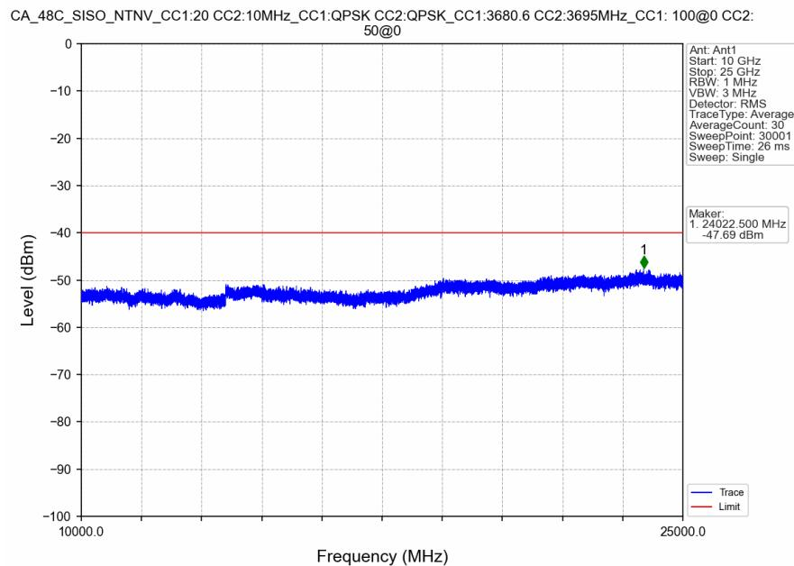
CA\_48C\_SISO\_NTNV\_CC1:20 CC2:10MHz\_CC1:QPSK CC2:QPSK\_CC1:3680.6 CC2:3695MHz\_CC1: 100@0 CC2:
