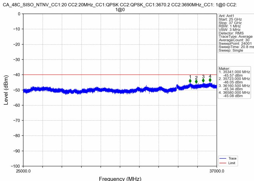
CA\_48C\_SISO\_NTNV\_CC1:20 CC2:20MHz\_CC1:QPSK CC2:QPSK\_CC1:3670.2 CC2:3690MHz\_CC1:1@99 CC2:1@99
