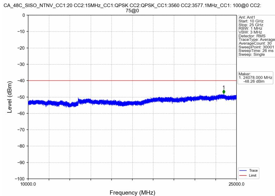
CA\_48C\_SISO\_NTNV\_CC1:20 CC2:15MHz\_CC1:QPSK CC2:QPSK\_CC1:3560 CC2:3577.1MHz\_CC1: 100@0 CC2:
