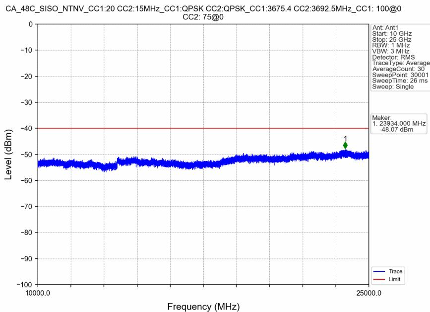
CA\_48C\_SISO\_NTNV\_CC1:20 CC2:15MHz\_CC1:QPSK CC2:QPSK\_CC1:3675.4 CC2:3692.5MHz\_CC1: 100@0 CC2: 75@0
