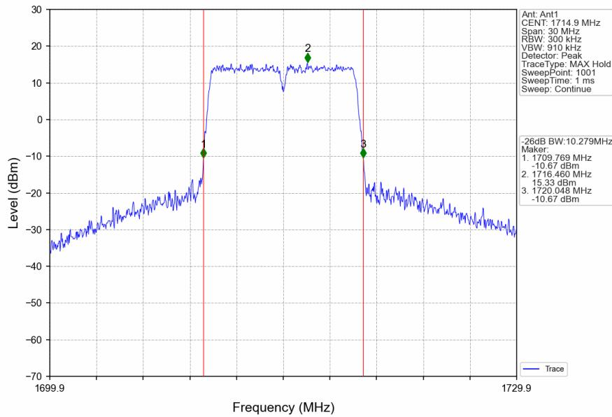
CA\_66B\_SISO\_NTNV\_CC1:5 CC2:5MHz\_CC1:16QAM CC2:16QAM\_CC1:1772.7 CC2:1777.5MHz\_CC1: 25@0 CC2: 25@0
