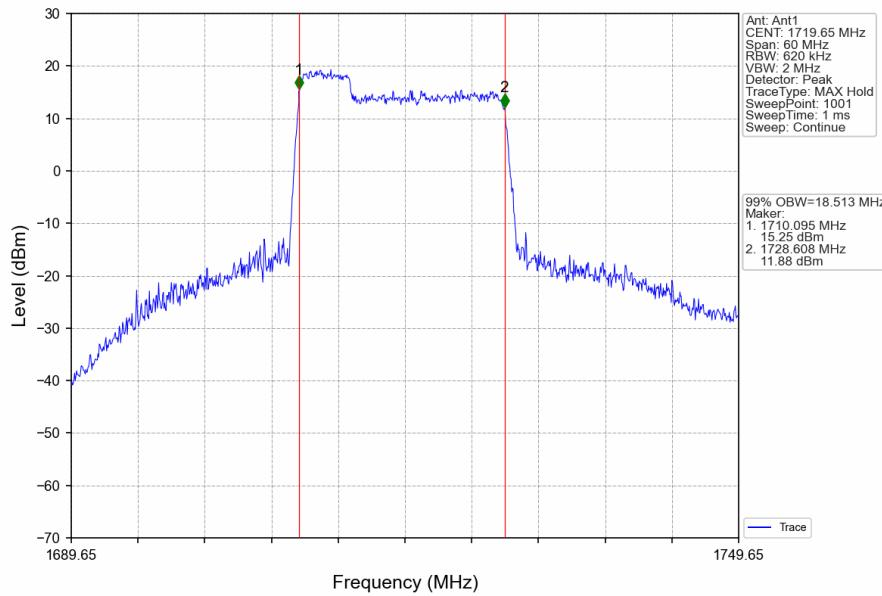
CA\_66B\_SISO\_NTNV\_CC1:5 CC2:15MHz\_CC1:16QAM CC2:16QAM\_CC1:1763.2 CC2:1772.5MHz\_CC1: 25@0 CC2: 75@0
