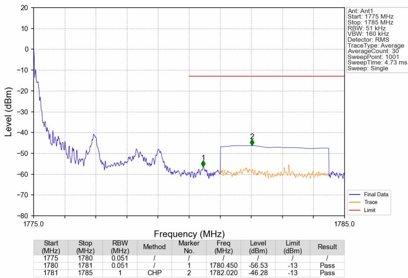
CA\_66B\_SISO\_NTNV\_CC1:5 CC2:5MHz\_CC1:QPSK CC2:QPSK\_CC1:1772.7 CC2:1777.5MHz\_CC1: 25@0 CC2:
