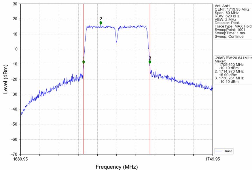
CA\_66B\_SISO\_NTNV\_CC1:10 CC2:10MHz\_CC1:QPSK CC2:QPSK\_CC1:1765.1 CC2:1775MHz\_CC1: 50@0 CC2:
