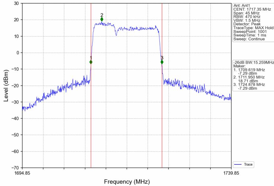
CA\_66B\_SISO\_NTNV\_CC1:5 CC2:10MHz\_CC1:16QAM CC2:16QAM\_CC1:1767.8 CC2:1775MHz\_CC1: 25@0 CC2: 50@0
