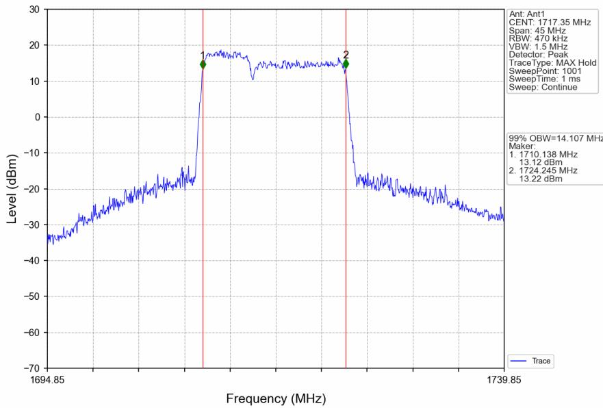
CA\_66B\_SISO\_NTNV\_CC1:5 CC2:10MHz\_CC1:16QAM CC2:16QAM\_CC1:1767.8 CC2:1775MHz\_CC1: 25@0 CC2: 50@0
