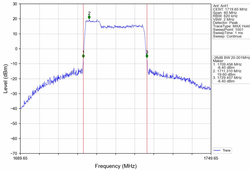
CA\_66B\_SISO\_NTNV\_CC1:5 CC2:15MHz\_CC1:QPSK CC2:QPSK\_CC1:1763.2 CC2:1772.5MHz\_CC1: 25@0 CC2: 75@0
