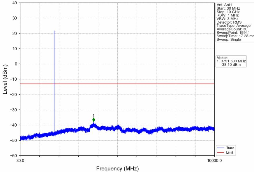
CA\_66B\_SISO\_NTNV\_CC1:5 CC2:5MHz\_CC1:QPSK CC2:QPSK\_CC1:1772.7 CC2:1777.5MHz\_CC1: 1@0 CC2: 1@0
