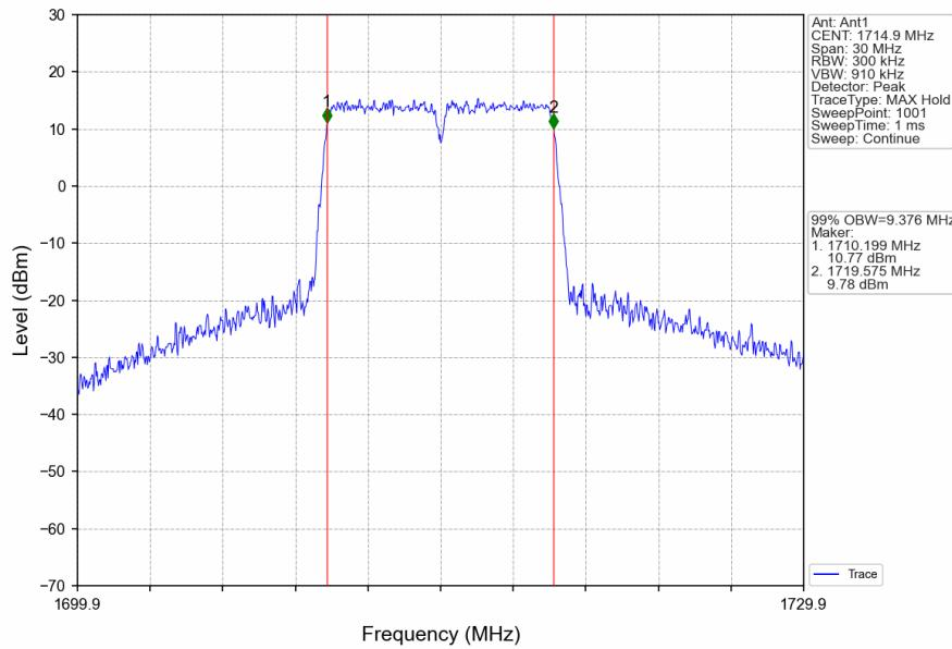
CA\_66B\_SISO\_NTNV\_CC1:5 CC2:5MHz\_CC1:16QAM CC2:16QAM\_CC1:1772.7 CC2:1777.5MHz\_CC1: 25@0 CC2: 25@0
