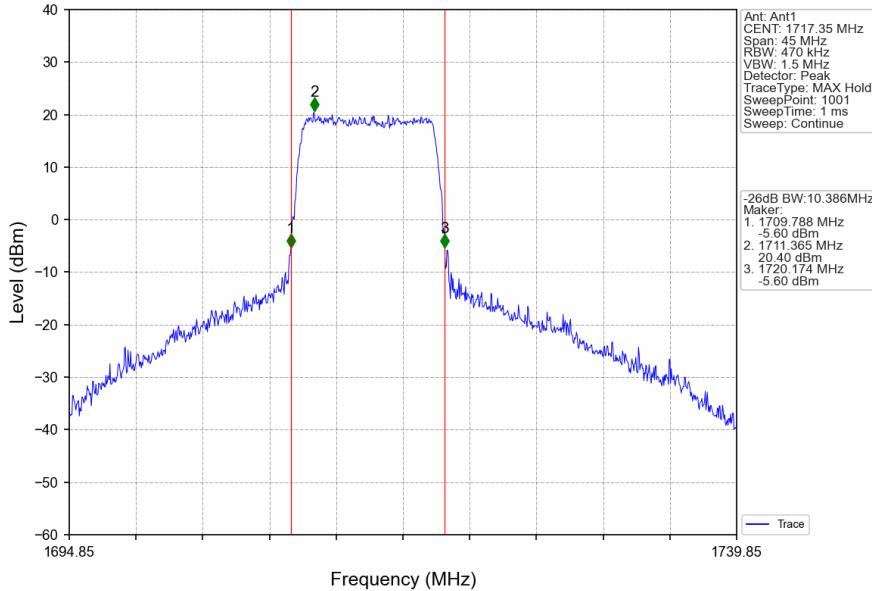
CA\_66B\_SISO\_NTNV\_CC1:10 CC2:5MHz\_CC1:QPSK CC2:QPSK\_CC1:1770.3 CC2:1777.5MHz\_CC1: 50@0 CC2: 25@0
