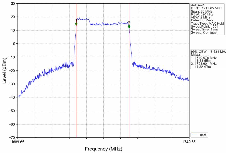
CA\_66B\_SISO\_NTNV\_CC1:5 CC2:15MHz\_CC1:QPSK CC2:QPSK\_CC1:1763.2 CC2:1772.5MHz\_CC1: 25@0 CC2: 75@0
