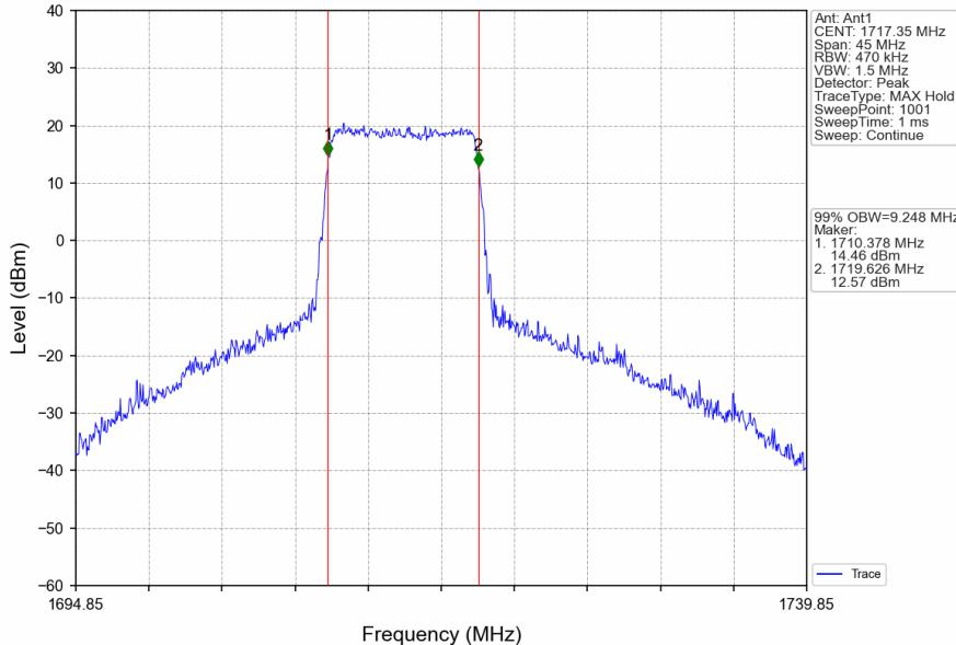
CA\_66B\_SISO\_NTNV\_CC1:10 CC2:5MHz\_CC1:QPSK CC2:QPSK\_CC1:1770.3 CC2:1777.5MHz\_CC1: 50@0 CC2: 25@0
