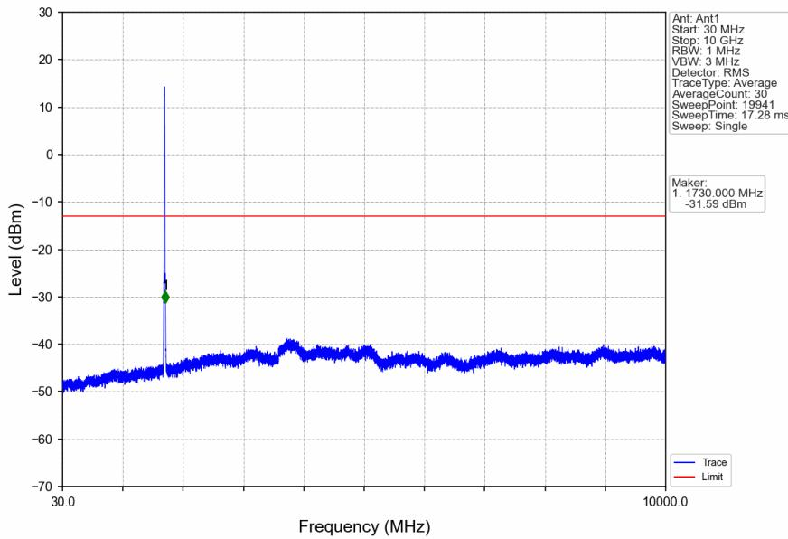
CA\_66B\_SISO\_NTNV\_CC1:5 CC2:5MHz\_CC1:QPSK CC2:QPSK\_CC1:1712.5 CC2:1717.3MHz\_CC1: 25@0 CC2:
