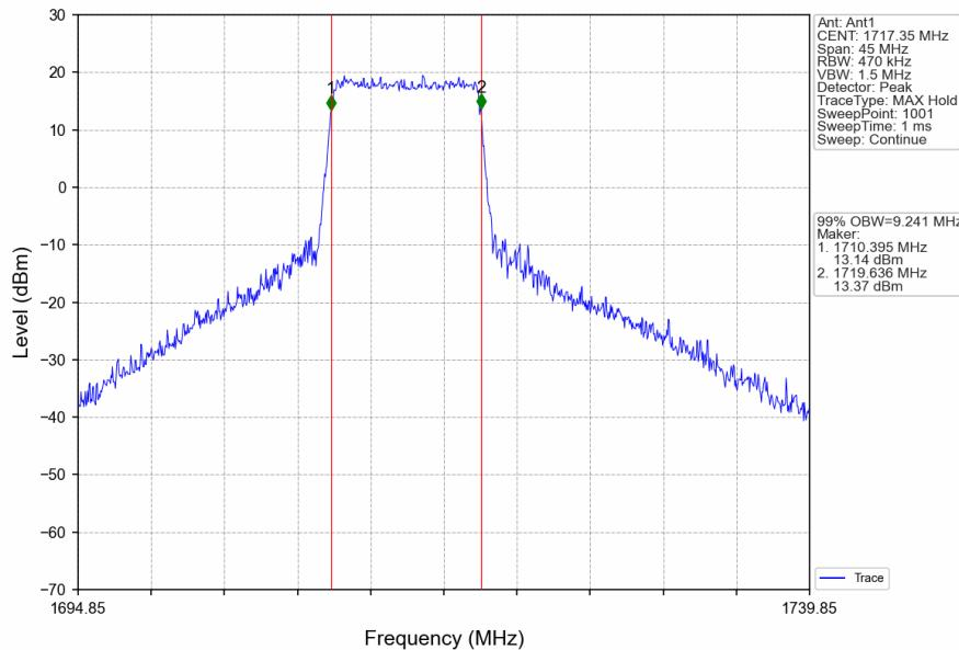
CA\_66B\_SISO\_NTNV\_CC1:10 CC2:5MHz\_CC1:16QAM CC2:16QAM\_CC1:1770.3 CC2:1777.5MHz\_CC1: 50@0 CC2: 25@0
