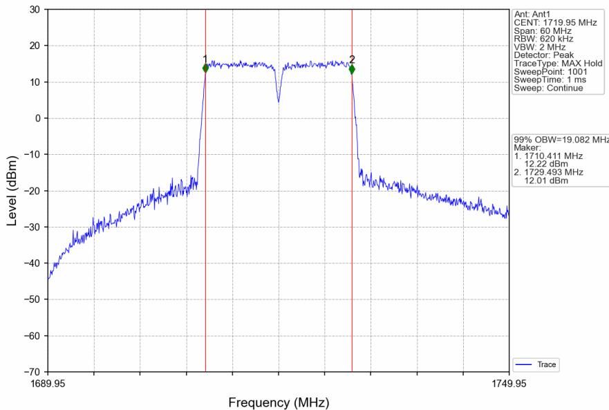
CA\_66B\_SISO\_NTNV\_CC1:10 CC2:10MHz\_CC1:QPSK CC2:QPSK\_CC1:1765.1 CC2:1775MHz\_CC1: 50@0 CC2:
