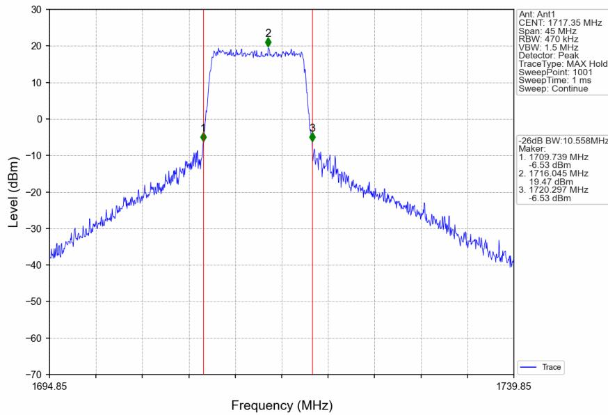
CA\_66B\_SISO\_NTNV\_CC1:10 CC2:5MHz\_CC1:16QAM CC2:16QAM\_CC1:1770.3 CC2:1777.5MHz\_CC1: 50@0 CC2: 25@0
