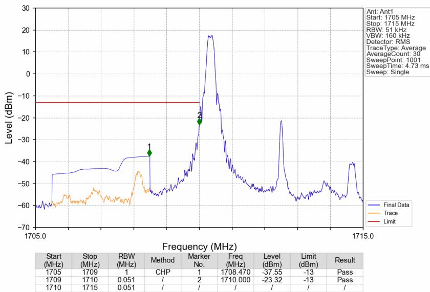
CA\_66B\_SISO\_NTNV\_CC1:5 CC2:5MHz\_CC1:16QAM CC2:16QAM\_CC1:1712.5 CC2:1717.3MHz\_CC1: 1@0 CC2: 1@0
