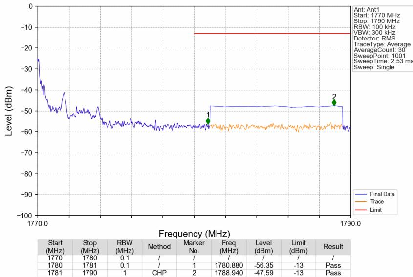
CA\_66B\_SISO\_NTNV\_CC1:10 CC2:10MHz\_CC1:QPSK CC2:QPSK\_CC1:1765.1 CC2:1775MHz\_CC1: 50@0 CC2:
