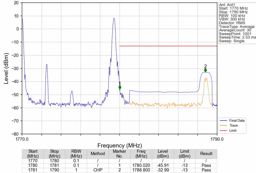
CA\_66B\_SISO\_NTNV\_CC1:5 CC2:10MHz\_CC1:QPSK CC2:QPSK\_CC1:1767.8 CC2:1775MHz\_CC1: 25@0 CC2: 50@0
