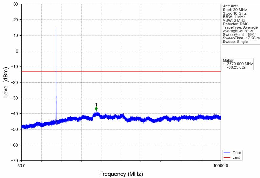
CA\_66B\_SISO\_NTNV\_CC1:10 CC2:5MHz\_CC1:16QAM CC2:16QAM\_CC1:1770.3 CC2:1777.5MHz\_CC1: 50@0 CC2: 25@0
