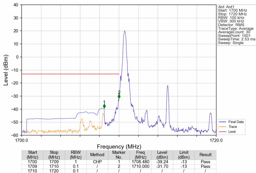
CA\_66B\_SISO\_NTNV\_CC1:10 CC2:10MHz\_CC1:16QAM CC2:16QAM\_CC1:1715 CC2:1724.9MHz\_CC1: 1@0 CC2: 1@0
