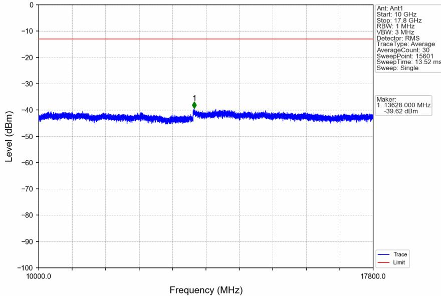
CA\_66B\_SISO\_NTNV\_CC1:10 CC2:5MHz\_CC1:QPSK CC2:QPSK\_CC1:1715 CC2:1722.2MHz\_CC1: 50@0 CC2: 25@0
