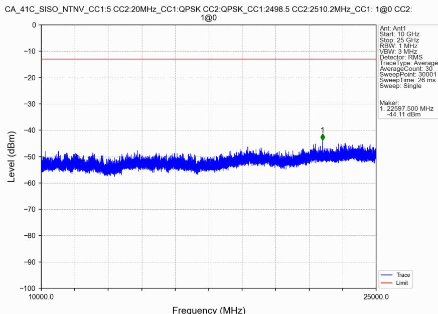
CA\_41C\_SISO\_NTNV\_CC1:5 CC2:20MHz\_CC1:QPSK CC2:QPSK\_CC1:2498.5 CC2:2510.2MHz\_CC1: 1@0 CC2: 1@0
