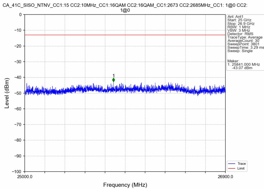
**CA\_41C\_SISO\_NTNV\_CC1:15 CC2:10MHz\_CC1:16QAM CC2:16QAM\_CC1:2673 CC2:2685MHz\_CC1: 1@74 CC2: 1@49**
