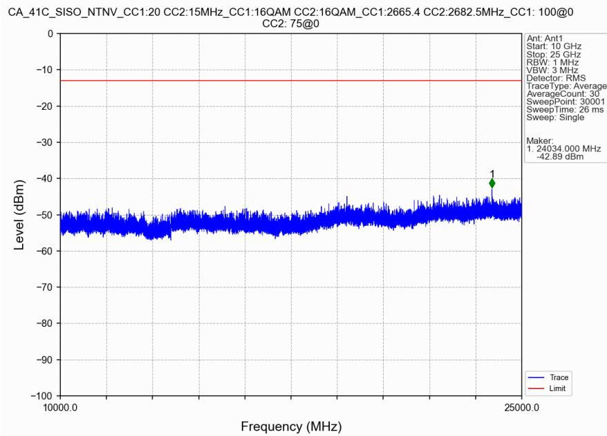
CA\_41C\_SISO\_NTNV\_CC1:20 CC2:15MHz\_CC1:16QAM CC2:16QAM\_CC1:2665.4 CC2:2682.5MHz\_CC1: 100@0
