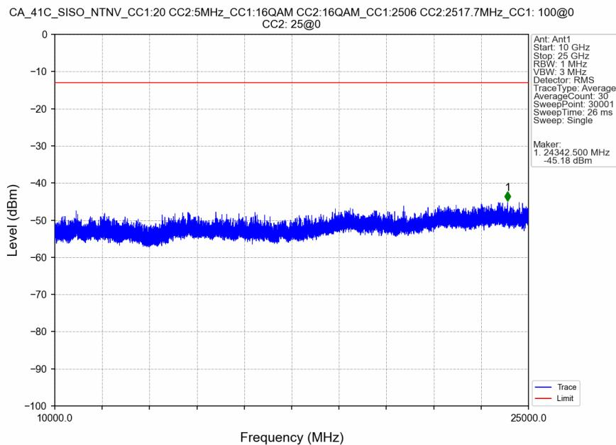
CA\_41C\_SISO\_NTNV\_CC1:20 CC2:5MHz\_CC1:16QAM CC2:16QAM\_CC1:2506 CC2:2517.7MHz\_CC1: 100@0 CC2: 25@0
