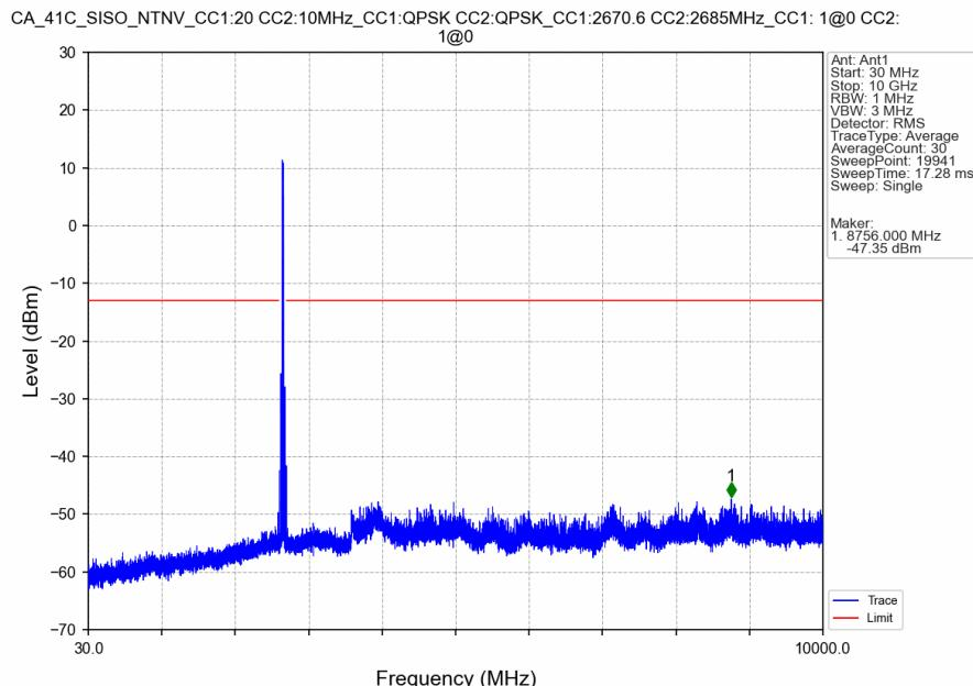
CA\_41C\_SISO\_NTNV\_CC1:20 CC2:10MHz\_CC1:QPSK CC2:QPSK\_CC1:2670.6 CC2:2685MHz\_CC1: 1@0 CC2: 1@0
