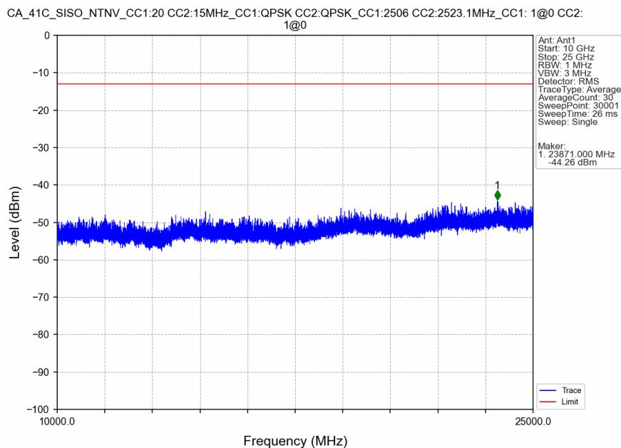
CA\_41C\_SISO\_NTNV\_CC1:20 CC2:15MHz\_CC1:QPSK CC2:QPSK\_CC1:2506 CC2:2523.1MHz\_CC1: 1@0 CC2: 1@0
