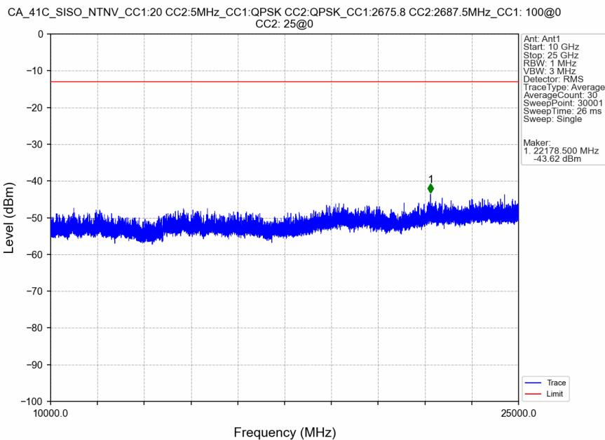
CA\_41C\_SISO\_NTNV\_CC1:20 CC2:5MHz\_CC1:QPSK CC2:QPSK\_CC1:2675.8 CC2:2687.5MHz\_CC1: 100@0 CC2:
