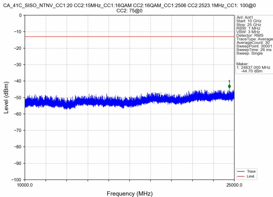
CA\_41C\_SISO\_NTNV\_CC1:20 CC2:15MHz\_CC1:16QAM CC2:16QAM\_CC1:2506 CC2:2523.1MHz\_CC1: 100@0
