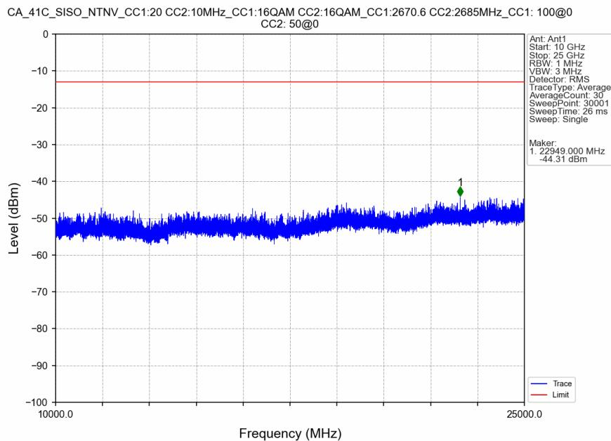
CA\_41C\_SISO\_NTNV\_CC1:20 CC2:10MHz\_CC1:16QAM CC2:16QAM\_CC1:2670.6 CC2:2685MHz\_CC1: 100@0
