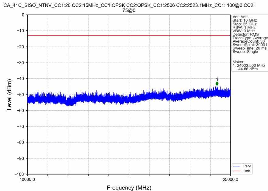
CA\_41C\_SISO\_NTNV\_CC1:20 CC2:15MHz\_CC1:QPSK CC2:QPSK\_CC1:2506 CC2:2523.1MHz\_CC1: 100@0 CC2:
