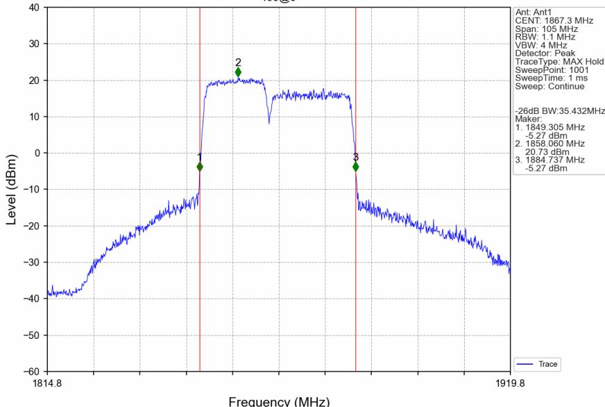
CA\_2C\_SISO\_NTNV\_CC1:15 CC2:20MHz\_CC1:QPSK CC2:QPSK\_CC1:1882.9 CC2:1900MHz\_CC1: 75@0 CC2:
