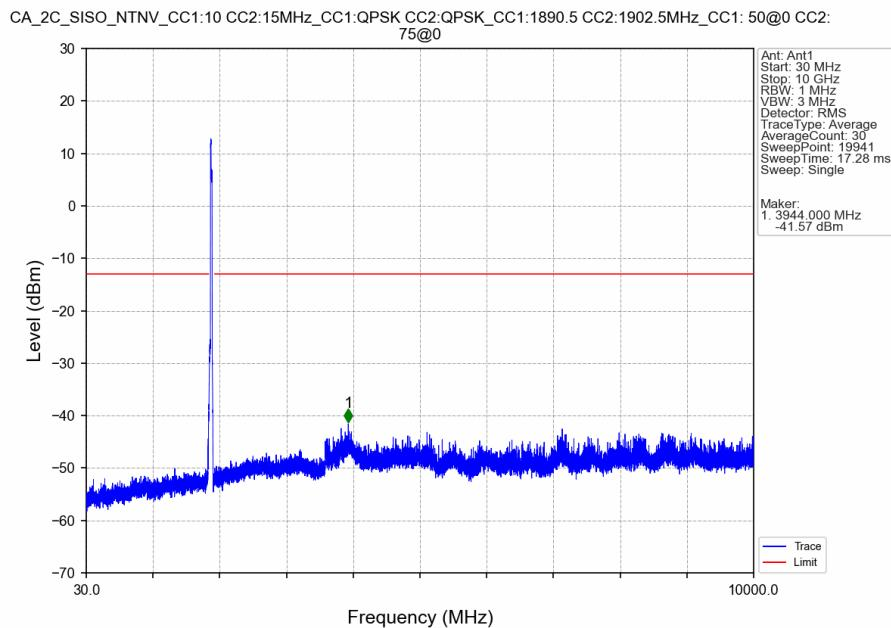
CA\_2C\_SISO\_NTNV\_CC1:10 CC2:15MHz\_CC1:QPSK CC2:QPSK\_CC1:1890.5 CC2:1902.5MHz\_CC1: 50@0 CC2: 75@0
