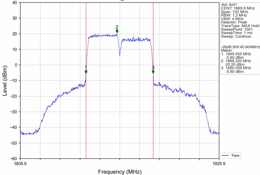
CA\_2C\_SISO\_NTNV\_CC1:20 CC2:20MHz\_CC1:QPSK CC2:QPSK\_CC1:1880.2 CC2:1900MHz\_CC1: 100@0 CC2: 100@0
