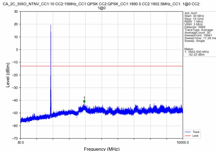
CA\_2C\_SISO\_NTNV\_CC1:10 CC2:15MHz\_CC1:QPSK CC2:QPSK\_CC1:1890.5 CC2:1902.5MHz\_CC1: 1@0 CC2: 1@0
