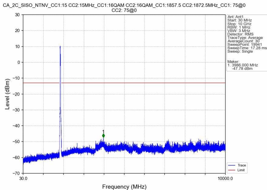
CA\_2C\_SISO\_NTNV\_CC1:15 CC2:15MHz\_CC1:16QAM CC2:16QAM\_CC1:1857.5 CC2:1872.5MHz\_CC1: 75@0 CC2: 75@0
