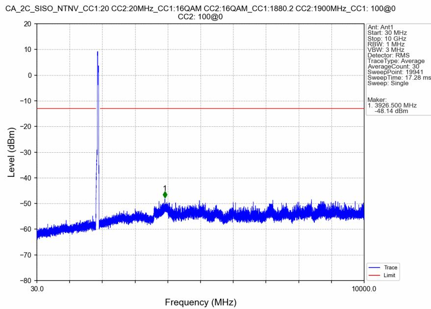
CA\_2C\_SISO\_NTNV\_CC1:20 CC2:20MHz\_CC1:16QAM CC2:16QAM\_CC1:1880.2 CC2:1900MHz\_CC1: 100@0 CC2: 100@0
