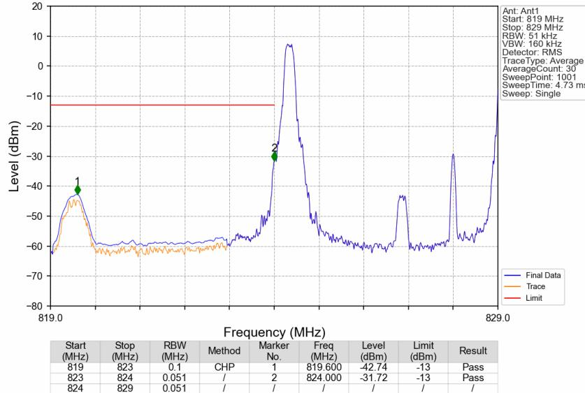
CA\_5B\_SISO\_NTNV\_CC1:5 CC2:3MHz\_CC1:QPSK CC2:QPSK\_CC1:826.5 CC2:830.4MHz\_CC1: 1@0 CC2: 1@0
