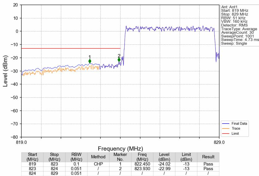
CA\_5B\_SISO\_NTNV\_CC1:5 CC2:3MHz\_CC1:16QAM CC2:16QAM\_CC1:826.5 CC2:830.4MHz\_CC1: 25@0 CC2: 15@0
