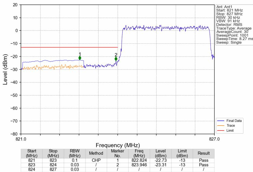
CA\_5B\_SISO\_NTNV\_CC1:3 CC2:5MHz\_CC1:16QAM CC2:16QAM\_CC1:825.5 CC2:829.4MHz\_CC1: 15@0 CC2: 25@0
