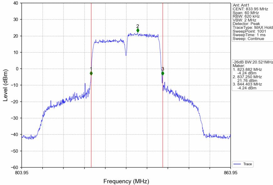
CA\_5B\_SISO\_NTNV\_CC1:10 CC2:10MHz\_CC1:QPSK CC2:QPSK\_CC1:834.1 CC2:844MHz\_CC1: 50@0 CC2: 50@0
