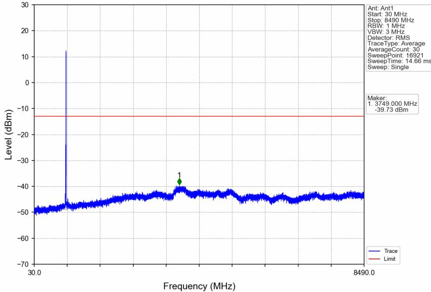
CA\_5B\_SISO\_NTNV\_CC1:5 CC2:3MHz\_CC1:QPSK CC2:QPSK\_CC1:843.6 CC2:847.5MHz\_CC1:1@24 CC2:1@14
