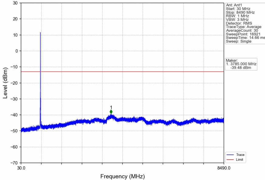
CA\_5B\_SISO\_NTNV\_CC1:5 CC2:10MHz\_CC1:QPSK CC2:QPSK\_CC1:836.8 CC2:844MHz\_CC1: 1@24 CC2: 1@49
