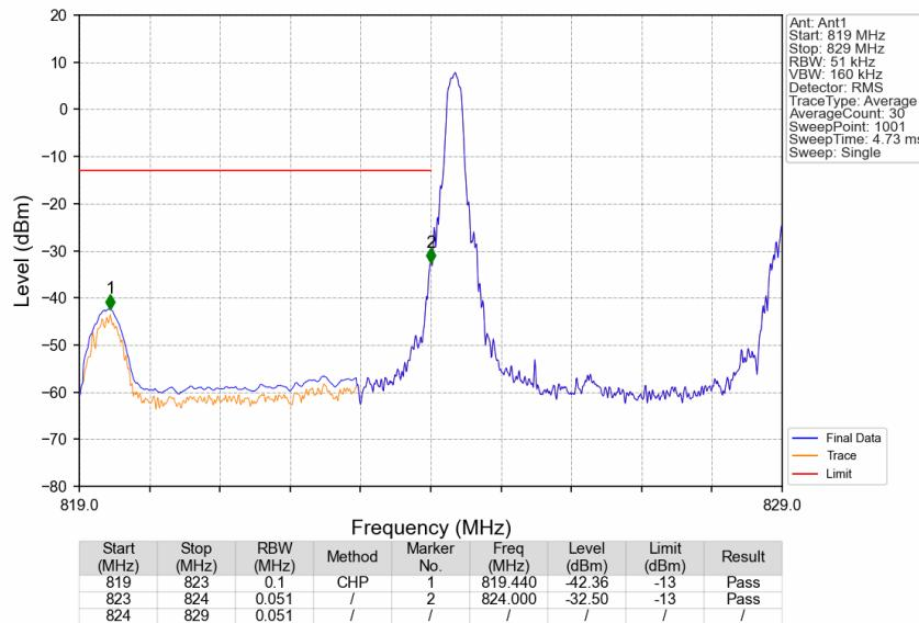
CA\_5B\_SISO\_NTNV\_CC1:5 CC2:10MHz\_CC1:QPSK CC2:QPSK\_CC1:826.5 CC2:833.7MHz\_CC1: 1@0 CC2: 1@0
