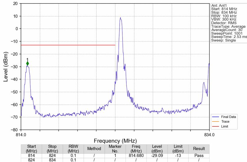
CA\_5B\_SISO\_NTNV\_CC1:10 CC2:10MHz\_CC1:QPSK CC2:QPSK\_CC1:829 CC2:838.9MHz\_CC1: 1@0 CC2: 1@0
