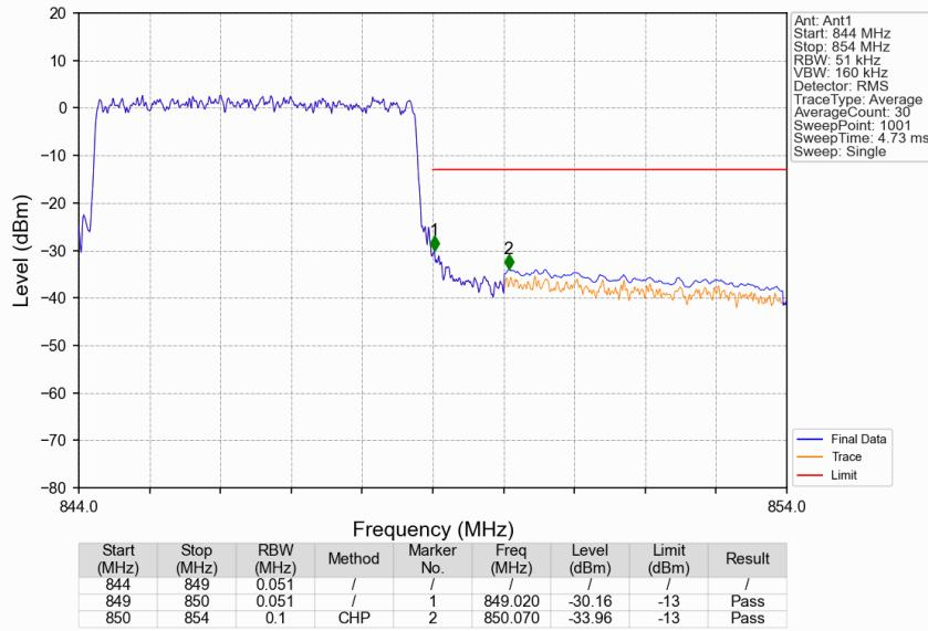
CA\_5B\_SISO\_NTNV\_CC1:10 CC2:5MHz\_CC1:QPSK CC2:QPSK\_CC1:839.3 CC2:846.5MHz\_CC1: 50@0 CC2: 25@0
