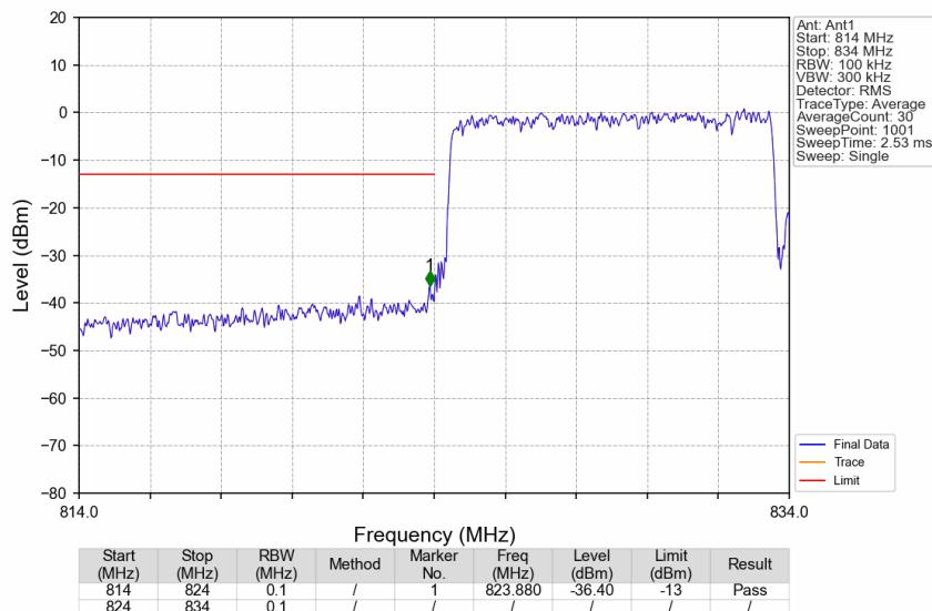
CA\_5B\_SISO\_NTNV\_CC1:10 CC2:10MHz\_CC1:16QAM CC2:16QAM\_CC1:829 CC2:838.9MHz\_CC1: 50@0 CC2:
