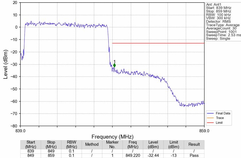
CA\_5B\_SISO\_NTNV\_CC1:10 CC2:10MHz\_CC1:QPSK CC2:QPSK\_CC1:834.1 CC2:844MHz\_CC1: 50@0 CC2: 50@0
