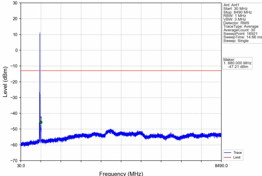
CA\_5B\_SISO\_NTNV\_CC1:10 CC2:10MHz\_CC1:16QAM CC2:16QAM\_CC1:834.1 CC2:844MHz\_CC1: 1@49 CC2: 1@49
