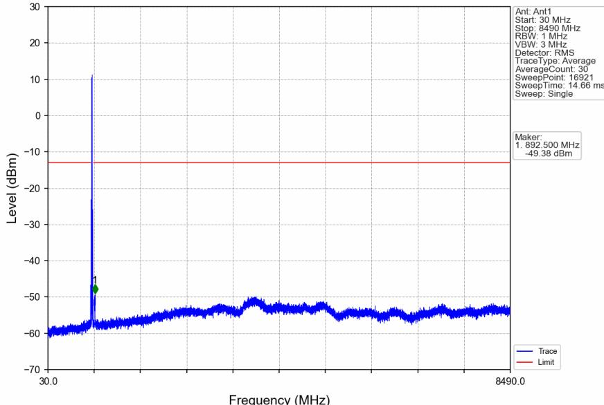
CA\_5B\_SISO\_NTNV\_CC1:10 CC2:10MHz\_CC1:QPSK CC2:QPSK\_CC1:834.1 CC2:844MHz\_CC1: 1@49 CC2: 1@49
