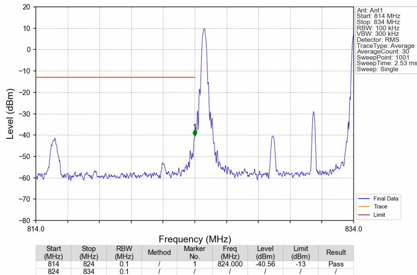
CA\_5B\_SISO\_NTNV\_CC1:10 CC2:5MHz\_CC1:QPSK CC2:QPSK\_CC1:829 CC2:836.2MHz\_CC1:1@0 CC2:1@0
