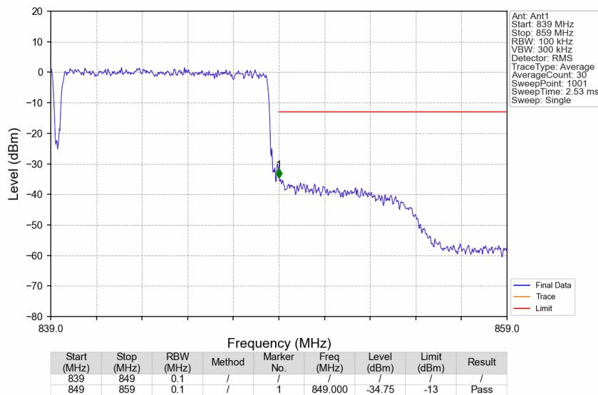
CA\_5B\_SISO\_NTNV\_CC1:5 CC2:10MHz\_CC1:16QAM CC2:16QAM\_CC1:836.8 CC2:844MHz\_CC1: 25@0 CC2:
