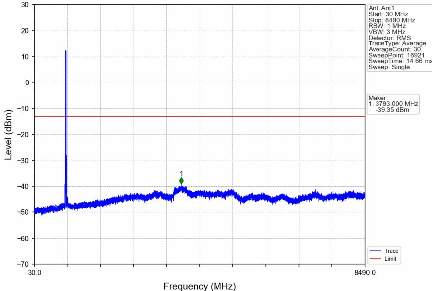
CA\_5B\_SISO\_NTNV\_CC1:10 CC2:5MHz\_CC1:QPSK CC2:QPSK\_CC1:839.3 CC2:846.5MHz\_CC1: 1@49 CC2: 1@24
