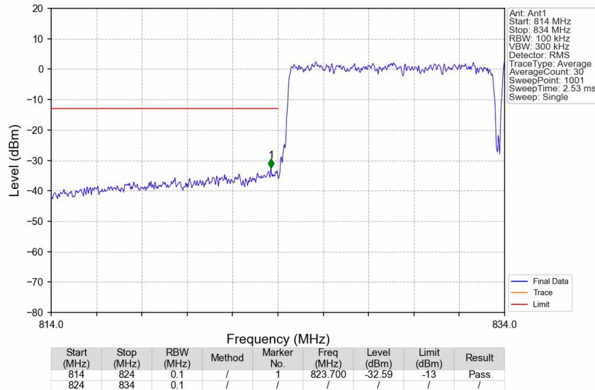
CA\_5B\_SISO\_NTNV\_CC1:10 CC2:5MHz\_CC1:QPSK CC2:QPSK\_CC1:829 CC2:836.2MHz\_CC1: 50@0 CC2: 25@0
