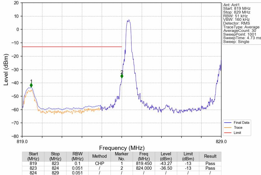
CA\_5B\_SISO\_NTNV\_CC1:5 CC2:10MHz\_CC1:16QAM CC2:16QAM\_CC1:826.5 CC2:833.7MHz\_CC1: 1@0 CC2: 1@0
