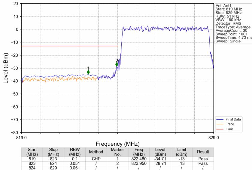
CA\_5B\_SISO\_NTNV\_CC1:5 CC2:10MHz\_CC1:QPSK CC2:QPSK\_CC1:826.5 CC2:833.7MHz\_CC1: 25@0 CC2: 50@0
