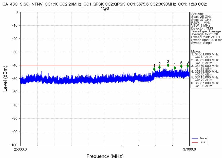
CA\_48C\_SISO\_NTNV\_CC1:10 CC2:20MHz\_CC1:QPSK CC2:QPSK\_CC1:3675.6 CC2:3690MHz\_CC1:1@49 CC2:1@99
