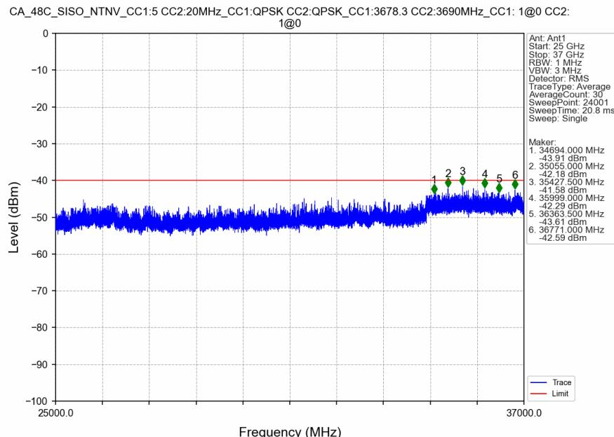
CA\_48C\_SISO\_NTNV\_CC1:5 CC2:20MHz\_CC1:QPSK CC2:QPSK\_CC1:3678.3 CC2:3690MHz\_CC1: 1@24 CC2: 1@99
