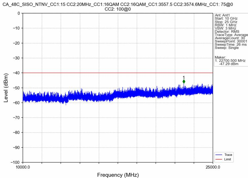
CA\_48C\_SISO\_NTNV\_CC1:15 CC2:20MHz\_CC1:16QAM CC2:16QAM\_CC1:3557.5 CC2:3574.6MHz\_CC1: 75@0
