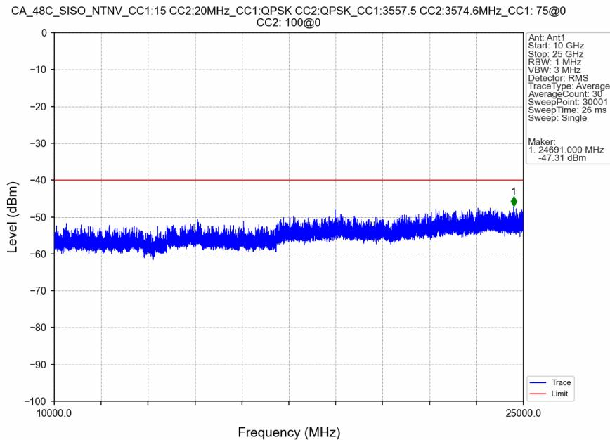
CA\_48C\_SISO\_NTNV\_CC1:15 CC2:20MHz\_CC1:QPSK CC2:QPSK\_CC1:3557.5 CC2:3574.6MHz\_CC1: 75@0 CC2: 100@0
