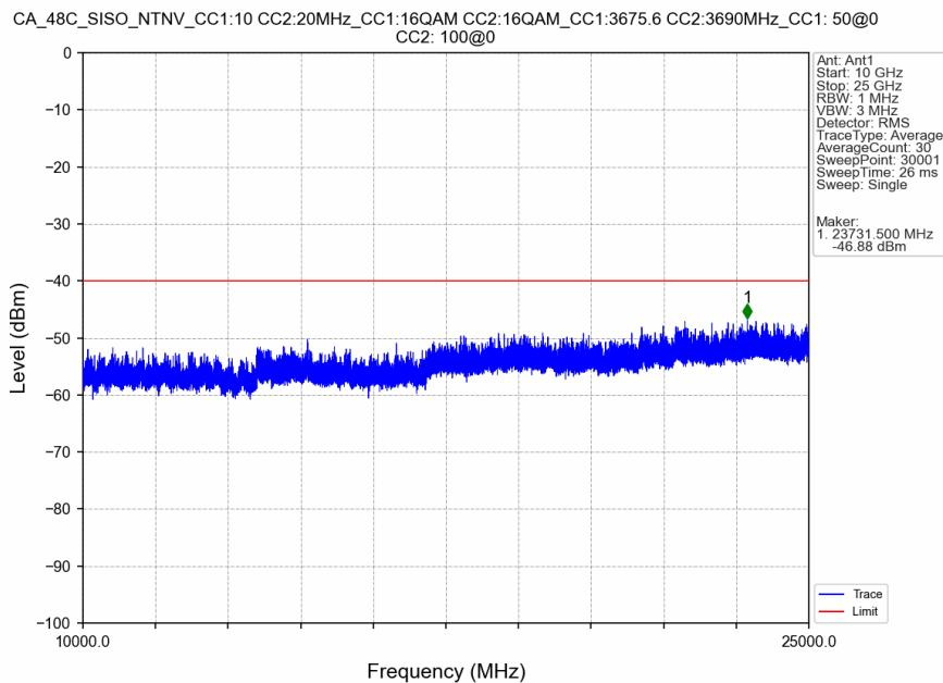
CA\_48C\_SISO\_NTNV\_CC1:10 CC2:20MHz\_CC1:16QAM CC2:16QAM\_CC1:3675.6 CC2:3690MHz\_CC1: 50@0 CC2: 100@0
