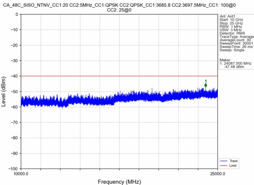
CA\_48C\_SISO\_NTNV\_CC1:20 CC2:5MHz\_CC1:QPSK CC2:QPSK\_CC1:3685.8 CC2:3697.5MHz\_CC1: 100@0 CC2:
