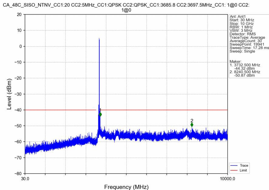
CA\_48C\_SISO\_NTNV\_CC1:20 CC2:5MHz\_CC1:QPSK CC2:QPSK\_CC1:3685.8 CC2:3697.5MHz\_CC1: 1@0 CC2: 1@0
