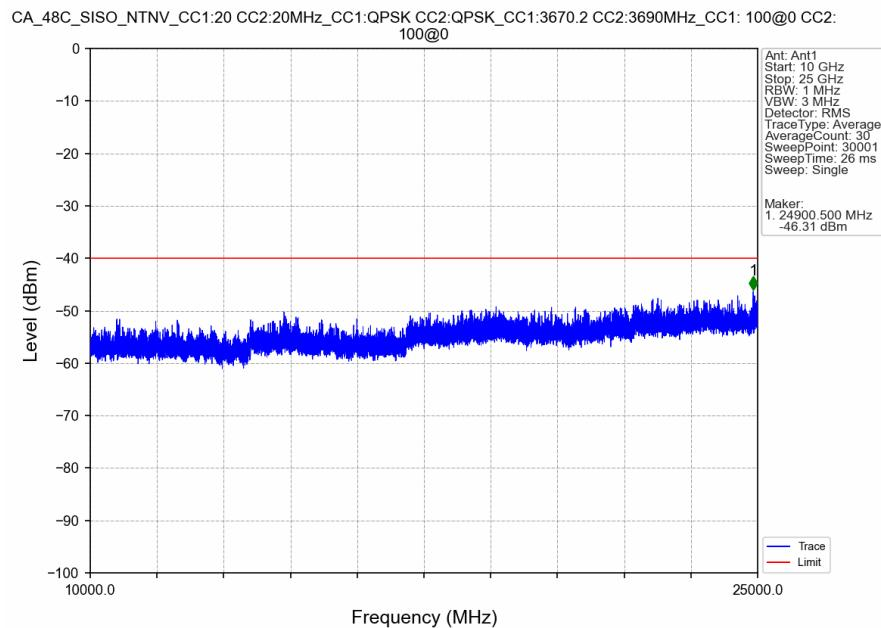
CA\_48C\_SISO\_NTNV\_CC1:20 CC2:20MHz\_CC1:QPSK CC2:QPSK\_CC1:3670.2 CC2:3690MHz\_CC1: 100@0 CC2:
