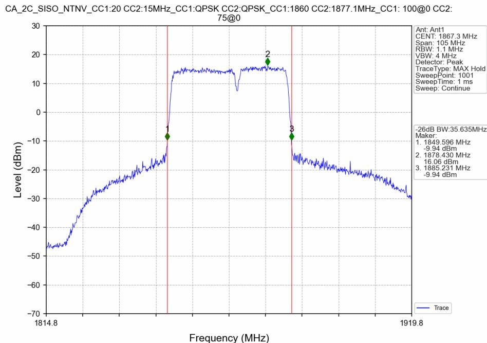
CA\_2C\_SISO\_NTNV\_CC1:20 CC2:15MHz\_CC1:QPSK CC2:QPSK\_CC1:1885.4
