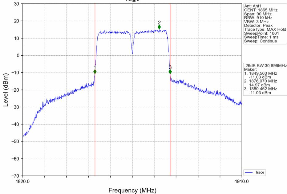
**CA\_2C\_SISO\_NTNV\_CC1:15 CC2:15MHz\_CC1:QPSK CC2:QPSK\_CC1:1887.5
