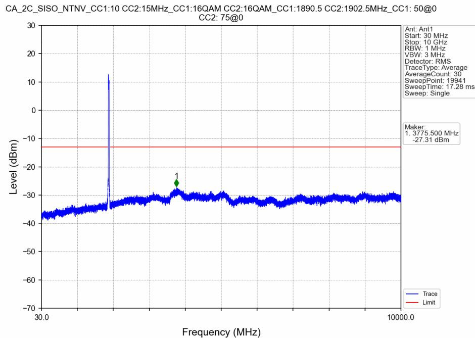
CA\_2C\_SISO\_NTNV\_CC1:10 CC2:15MHz\_CC1:16QAM CC2:16QAM\_CC1:1890.5
